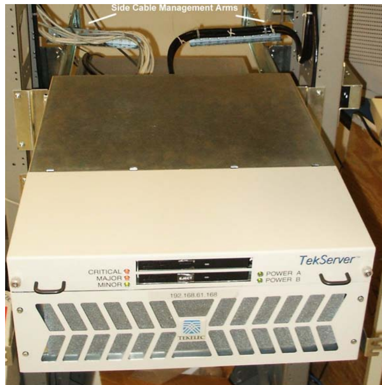
Figure 3-7. T1000 AS with Side Cable Management Arms
