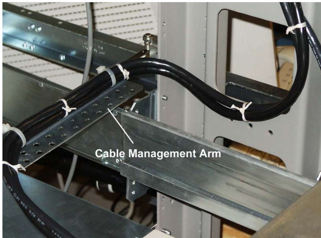
Figure 5-9. Detail of a Side Cable Management Arm
