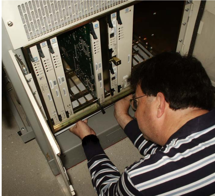
Figure 6-17. Insert fan tray bracket
