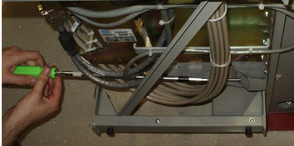
Figure 6-22. Tighten fan side bracket screws
