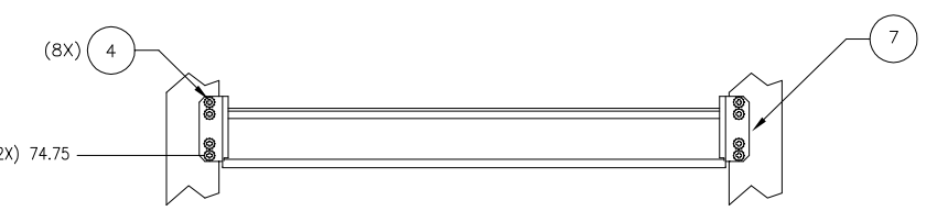
AIR DEFLECTOR POSITION, FRONT VIEW DETAIL C 4
