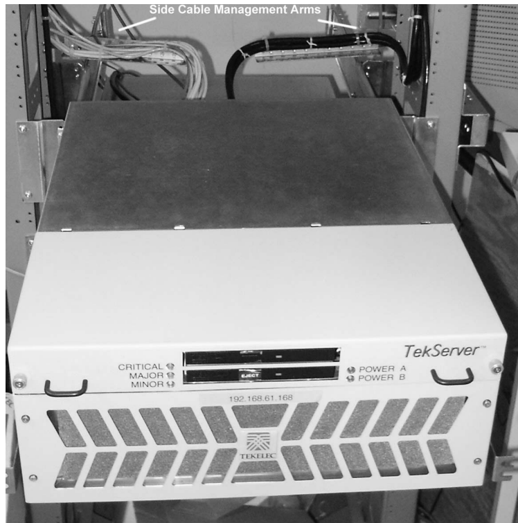
Figure 3-7. Tekelec 1000 with Side Cable Management Arms
