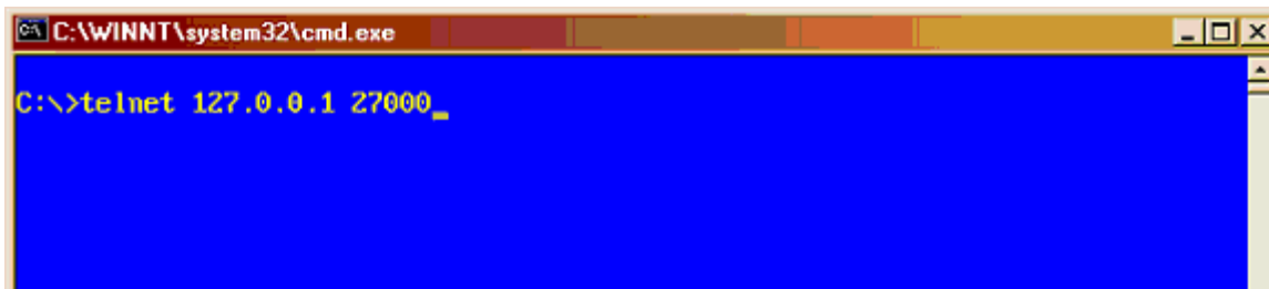
Figure B-9. Telnet Connection to Local Host Forwarded Port
