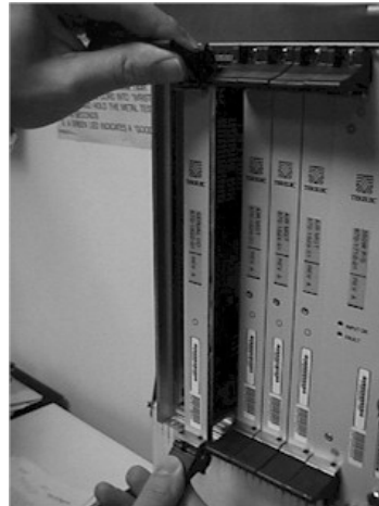
Figure 5-71. Freeing the Card from the EOAP Card Cage
