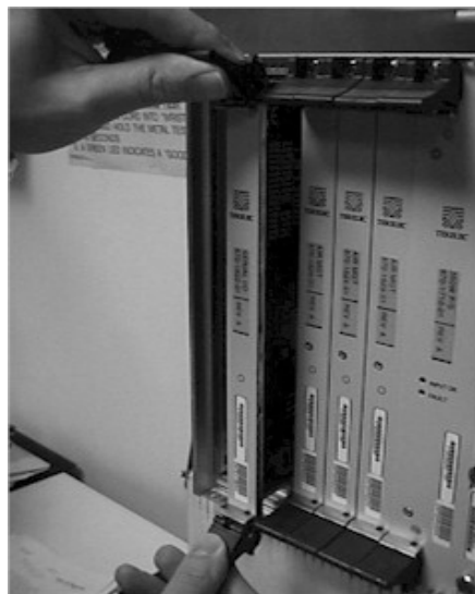
Figure 5-75. Inserting the Replacement Serial Card
