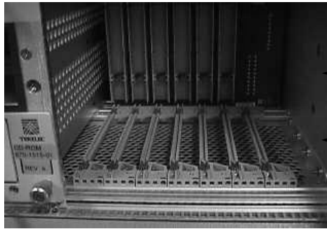
Figure 5-62. EOAP Backplane Connector Pins
