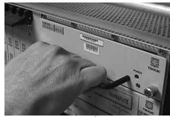
Figure 5-44. Free Hard Drive Card from the EOAP Card Cage
