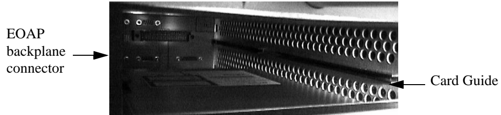
Figure 5-46. Examine EOAP Backplane Connector Pins
