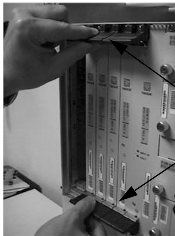
Figure 5-9. Lock the Inject/Eject Handles
