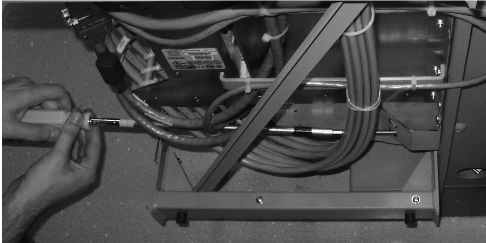
Figure A-28. Tighten fan side bracket screws
