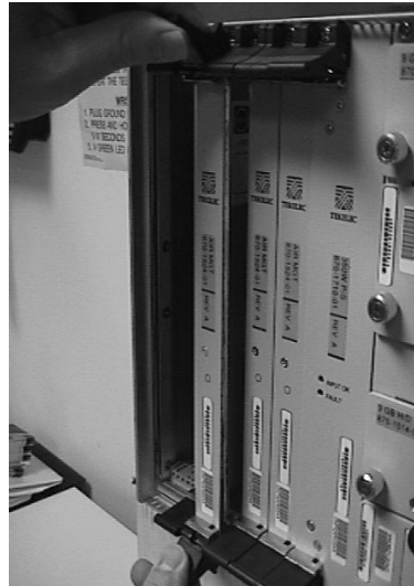
Figure 5-8. Inserting the Replacement Air Management Card
