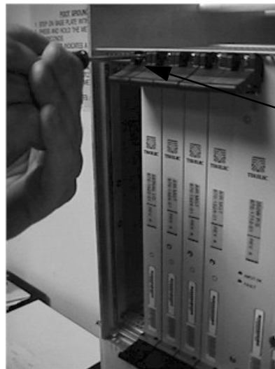
Figure 5-77. Tighten Captive Screws
