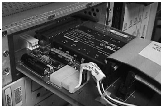
Figure 5-48. Installing the Hard Drive Card
