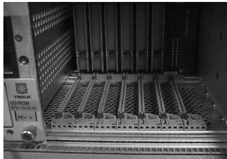
Figure 5-72. EOAP Backplane Connector Pins
