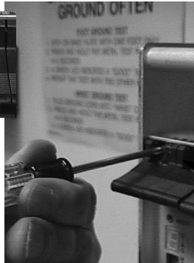
Figure 5-60. Processor Card Captive Screws
