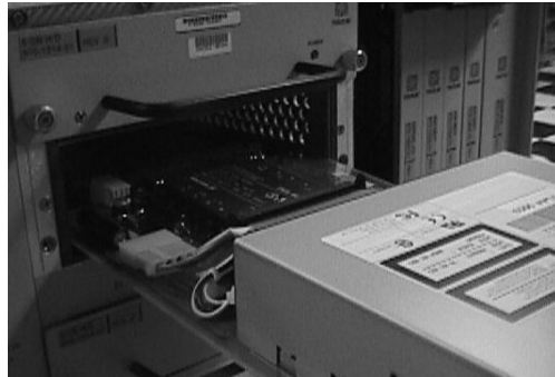
Figure 5-32. Install the CD-ROM Drive Card
