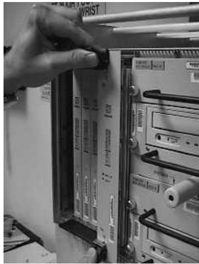
Figure 5-56. Inserting the Power Supply Card
