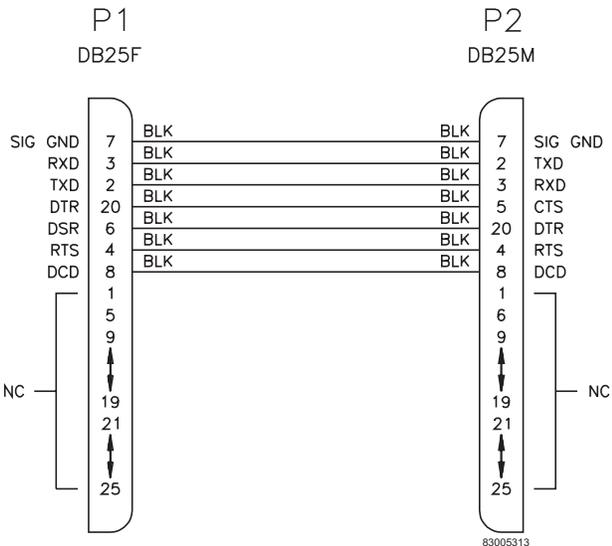
Serial Interface, Terminal, and Printer Adapter
