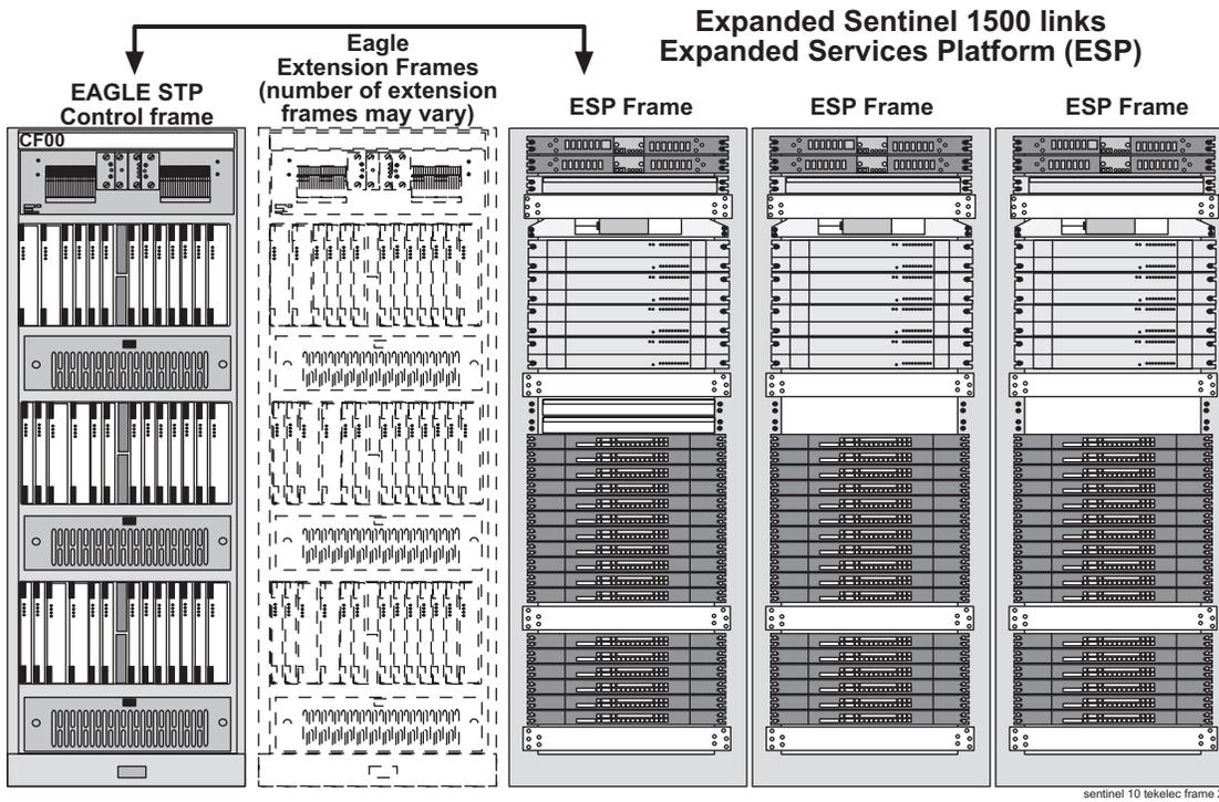
Figure 3-3 shows a maximum configuration front view of the Sentinel Processor Frame (SPF-00). 00 refers to the first Sentinel frame. Frame installation procedures are described in the *Tekelec 1000 Application Server Hardware Manual*.
