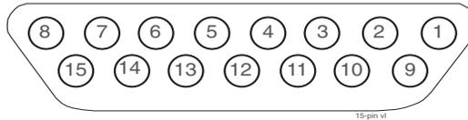
**Table B-35.** General Purpose Serial Interface Connector 01, GPSI
