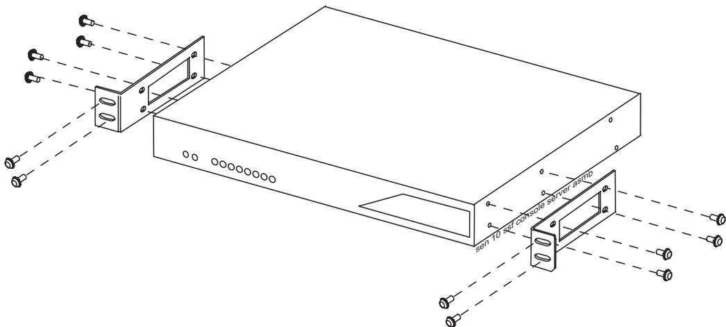
**Procedure — Mounting the Console Server**
