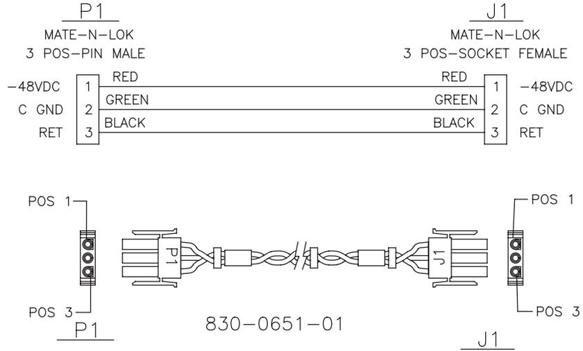
Power Cable (DC), Breaker Panel-to-Hub
