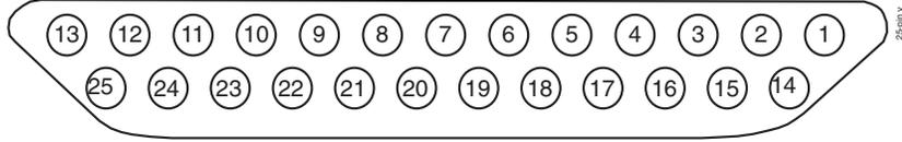
**Table B-17.** Clock B In Connector on Control Shelf backplane 04
