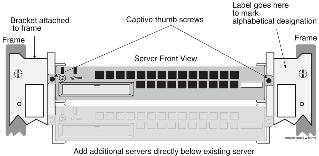
Place the next added server directly below the existing installed server using the Internal Frame Expansion Kit.
