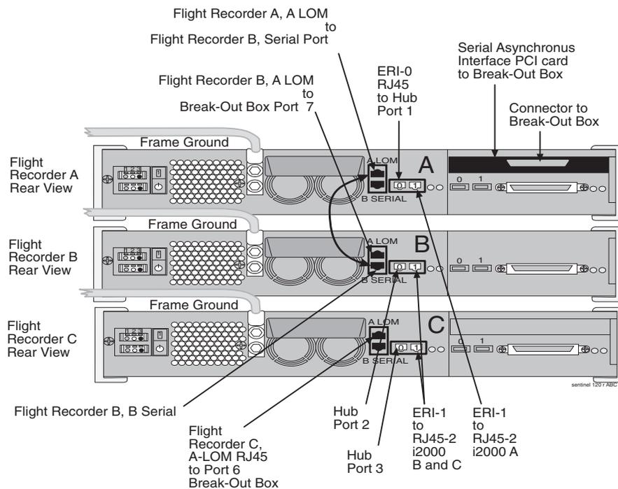
See Figure 3-13 for installation information on the flight recorders (model 120 servers).
