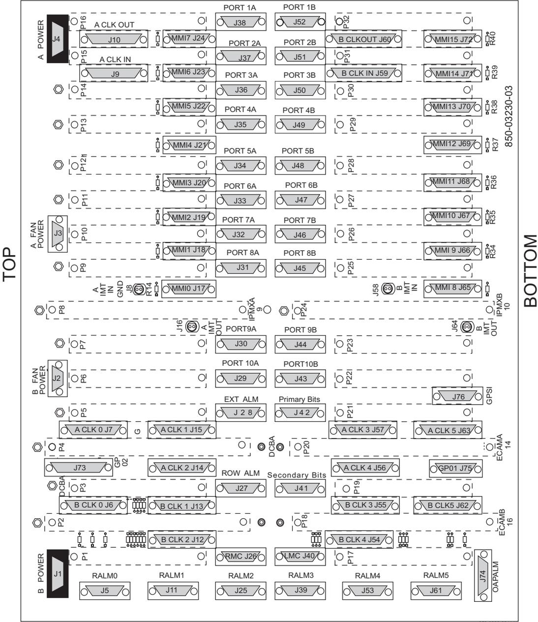
NOTE: Ⓞ Conducts -48VDC for the printed circuit board
