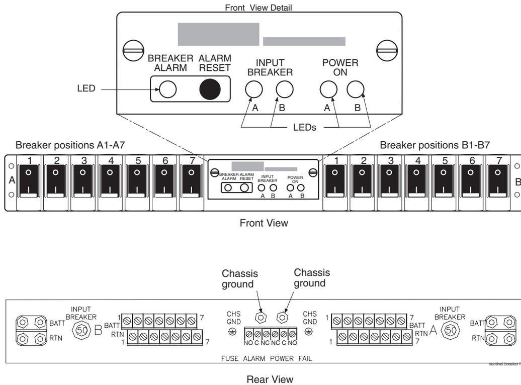
**NOTE:** When breakers trip to the half-way position as a result of an overload, they must be switched completely OFF, then ON to reset.
