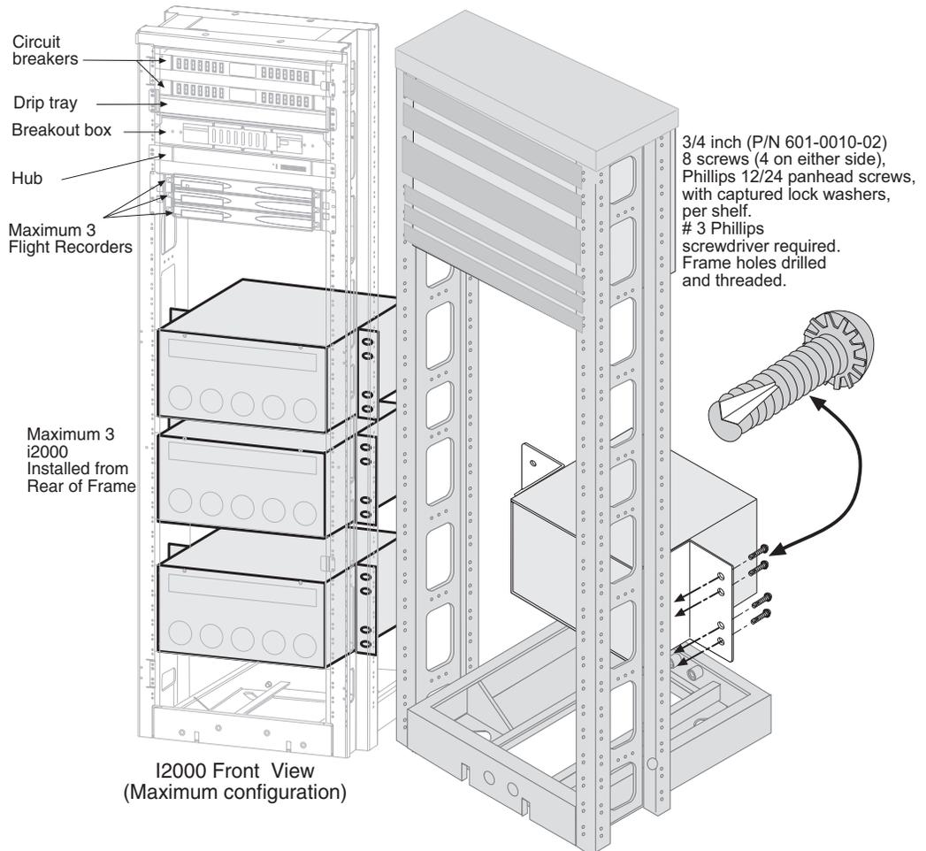
Figure 3-34. Site Collector Frame, Rear
