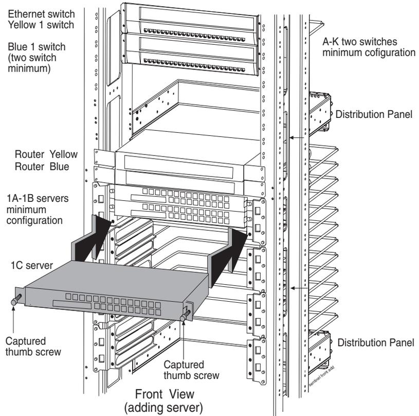
See Figure 3-15 for the location of the thumb screws.
