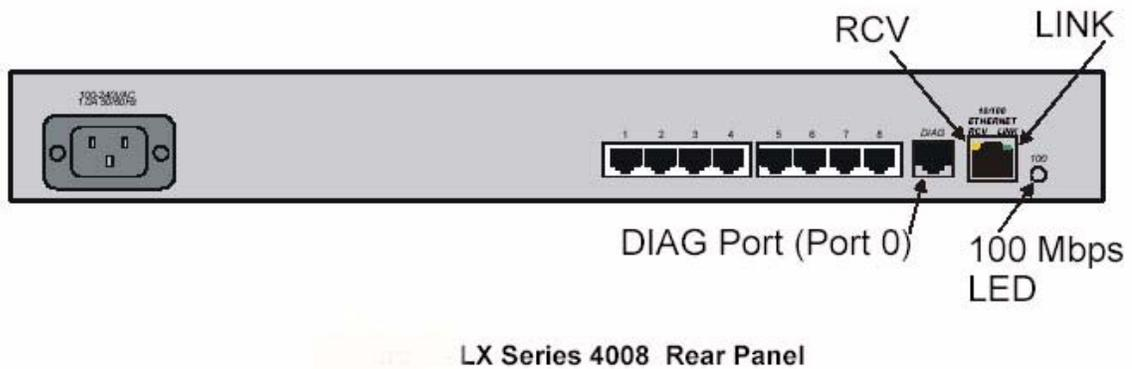
MRV™ Model LX Series 4008M with modem rear panel (console server) hardware in the Sentinel server frames that support Sentinel products.
