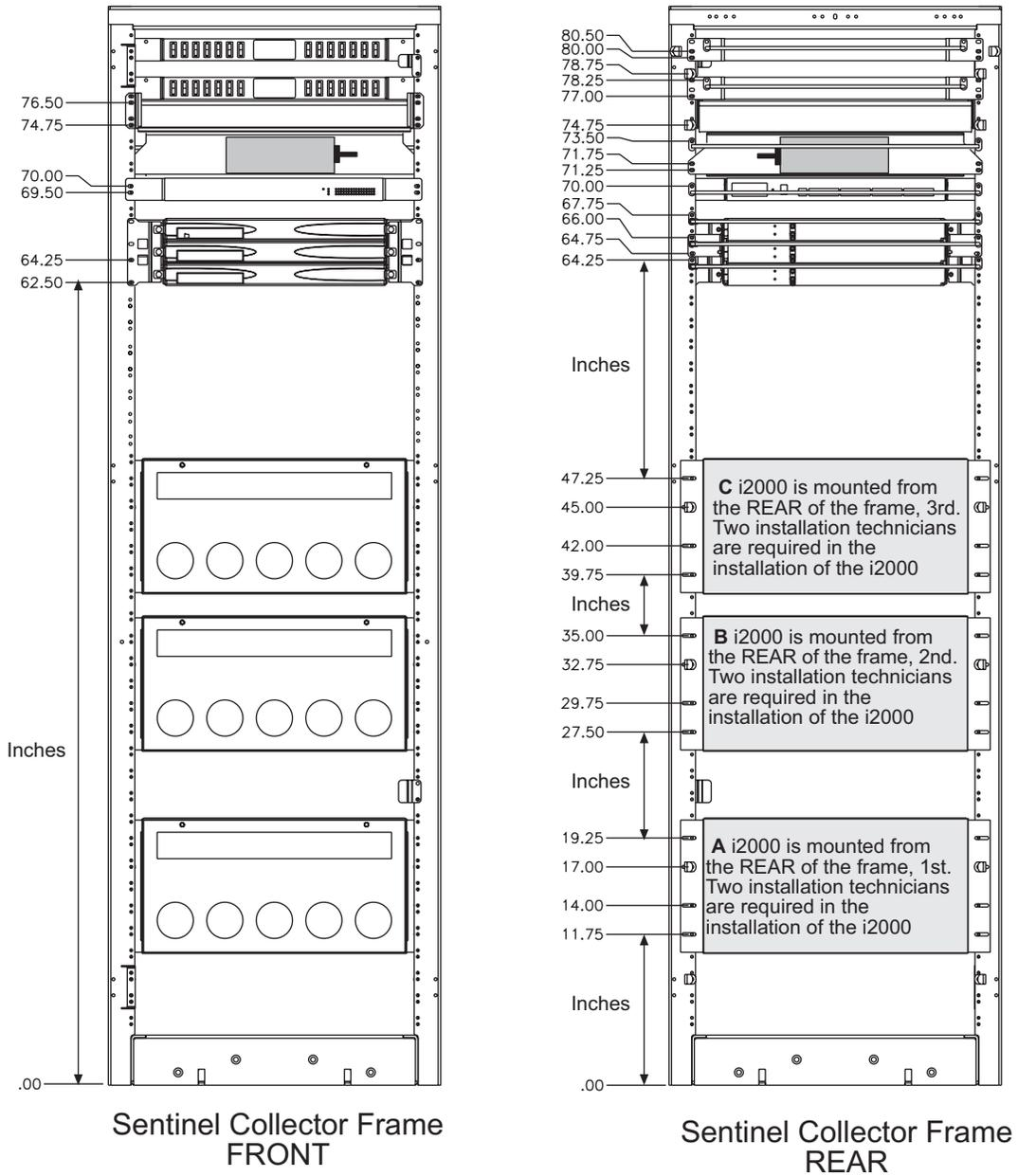
All measurements in Figure 3-26 are in inches. The i2000 shelf weighs approximately 44 kilos or 96.8lbs and requires two technicians to install it properly from the rear of the frame. Use four 12-24 0.75 inch (P/N 601-0010-02) screws, with a captive external tooth lock washers, on each side for a total of eight screws per shelf.
