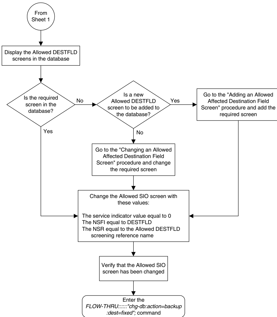
Flowchart 5-24. Changing an Allowed SIO Screen from the SEAS Terminal (Sheet 4 of 7)
