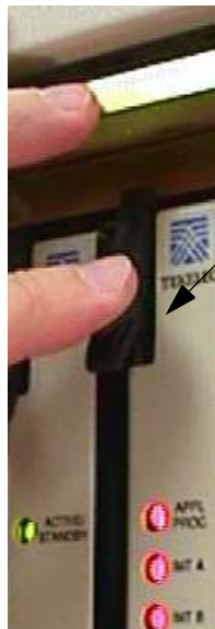
Figure 4-1. Push in Inject/Eject Clamp
