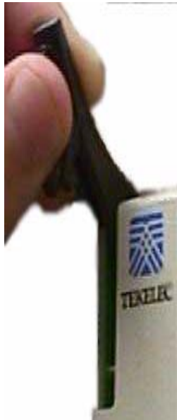
Figure 4-2. Push Inject/Eject Clamps Outward
