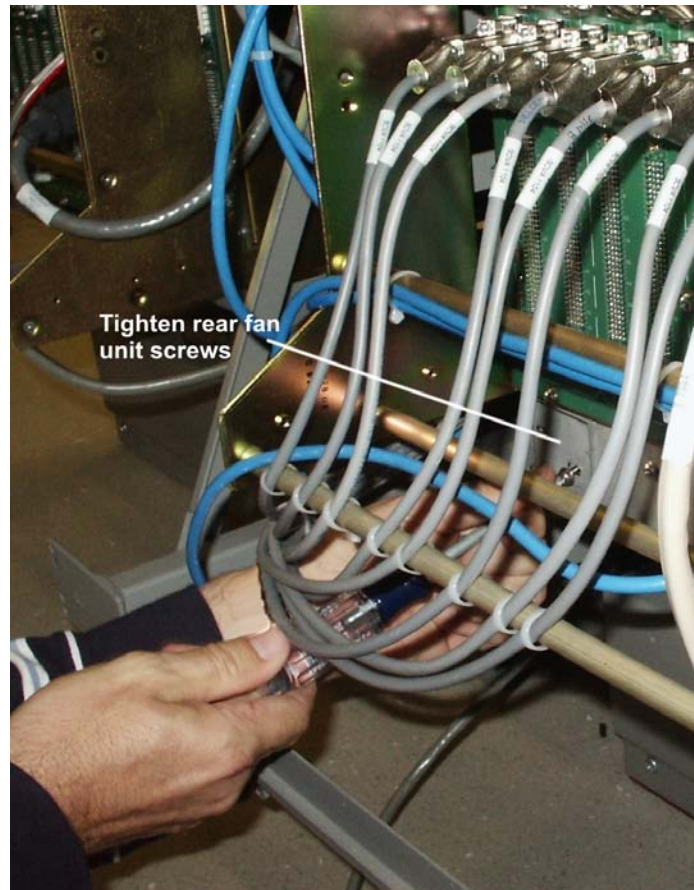
Figure A-29. Tighten rear fan tray screws
