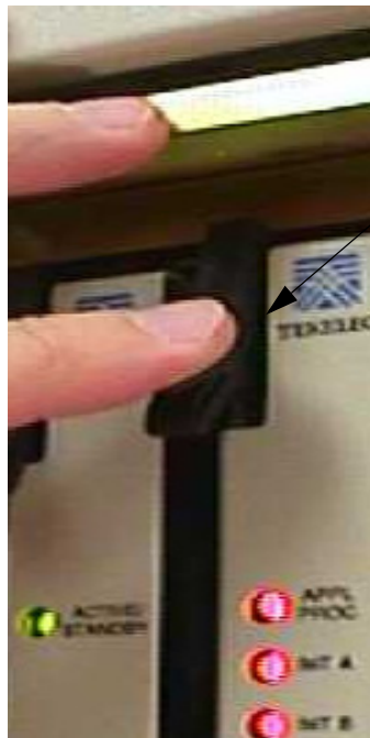
Figure 3-8. Push in Inject/Eject Clamps
