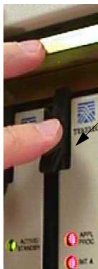
Figure A-18.Push in Inject/Eject Clamps
