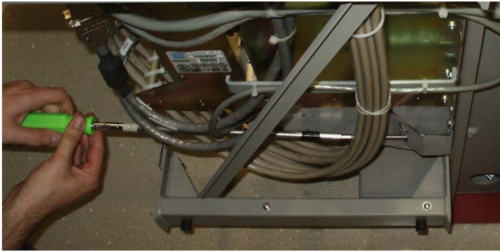
Figure A-30. Tighten fan side bracket screws
