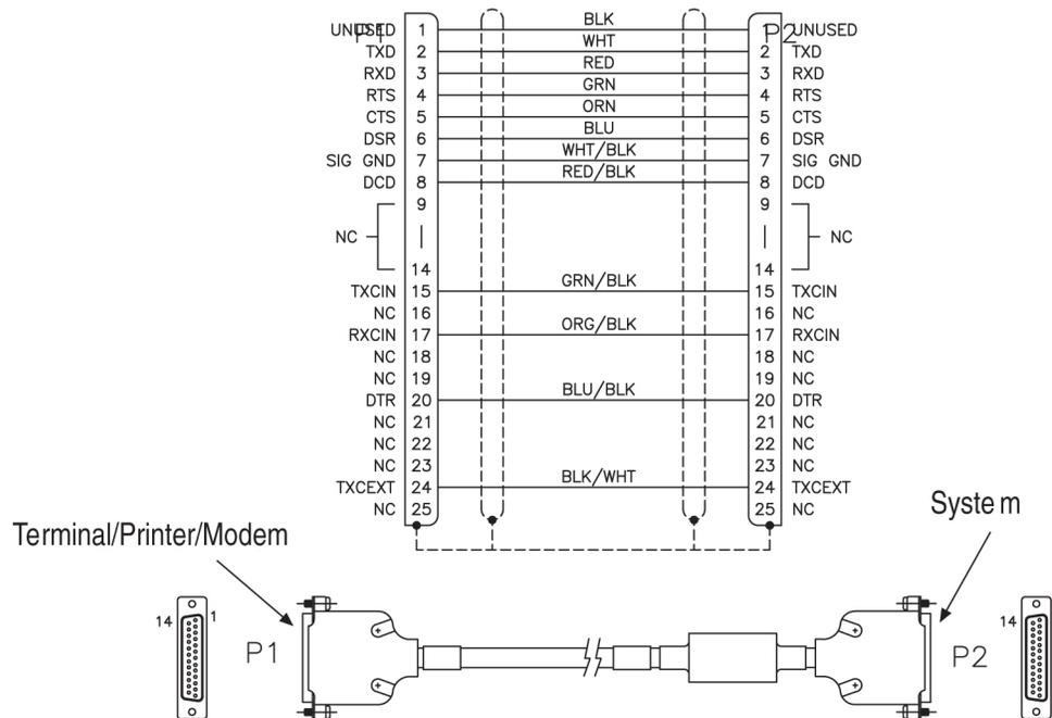
Figure 232: Modem/Terminal Cable
