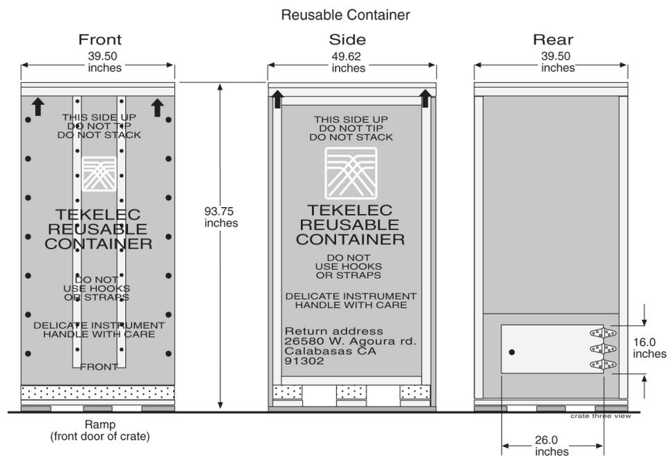
**Figure 9: Shipping Container for Heavy Duty Frame**
