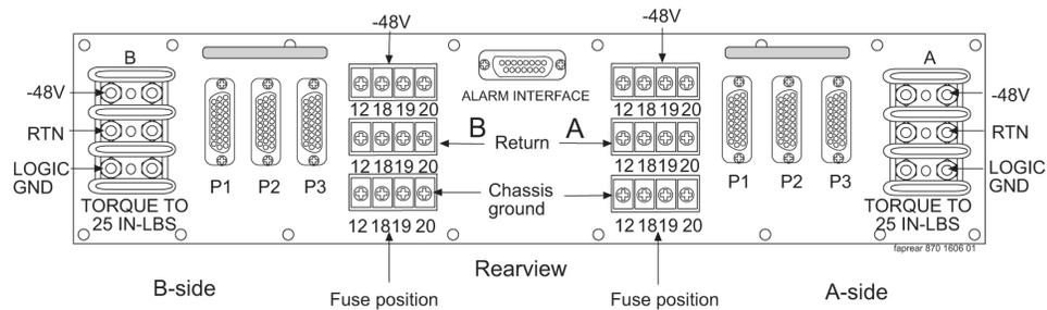
**Figure 50: 3U Fuse and Alarm Panel Rear (P/N 870-2320-03)**
