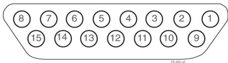
Figure 175: Serial Port Connector
