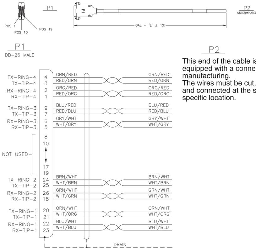
This end of the cable is not equipped with a connector in manufacturing. The wires must be cut, dressed, and connected at the site specific location.
