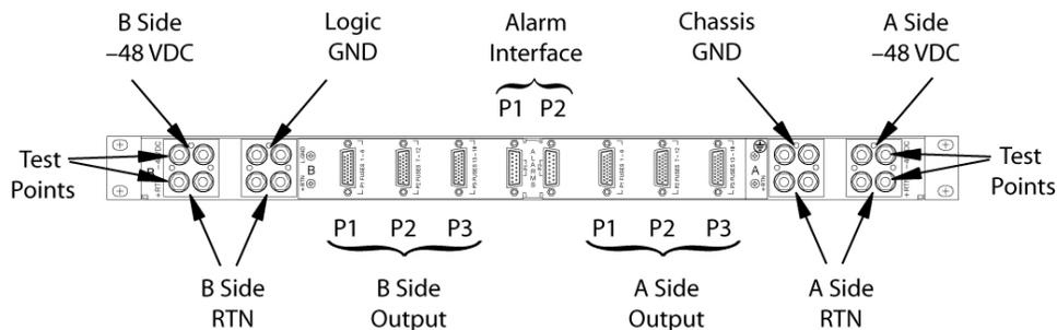
**Figure 49: 1U Fuse and Alarm Panel Rear (P/N 870-2804-01)**
