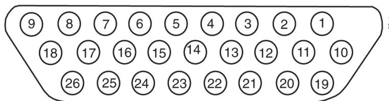
**Figure 166: External Alarm Connector**
