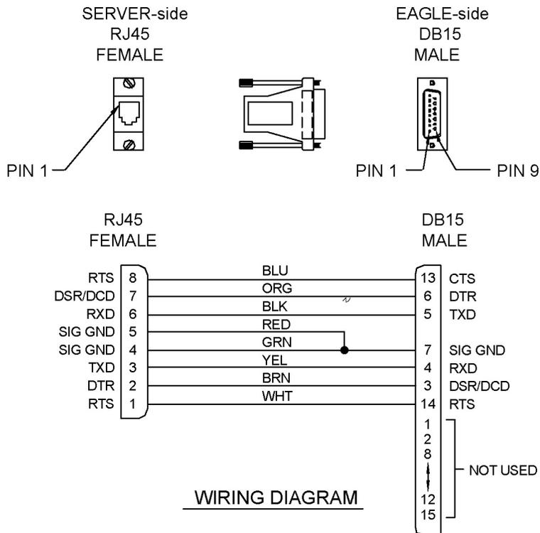
**Figure 259: Terminal/Server Serial Port Adapter, MRV (P/N 830-0915-02)**
