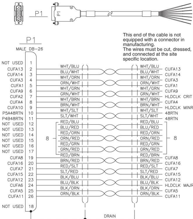
Figure 218: External Alarm Cable (Custom)
