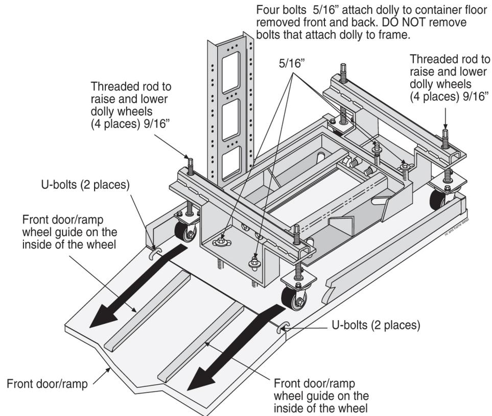
**Figure 11: Shipping, Detach Dolly Heavy Duty Frame**
