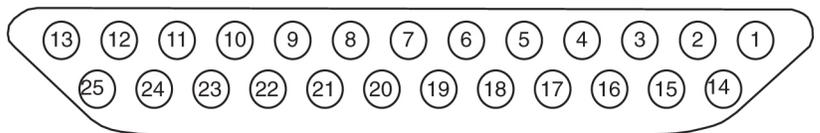
Figure 173: Clock B Out Connector on Backplane
