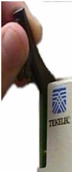
**Figure 79: Push Inject/Eject Clamps Outward**
