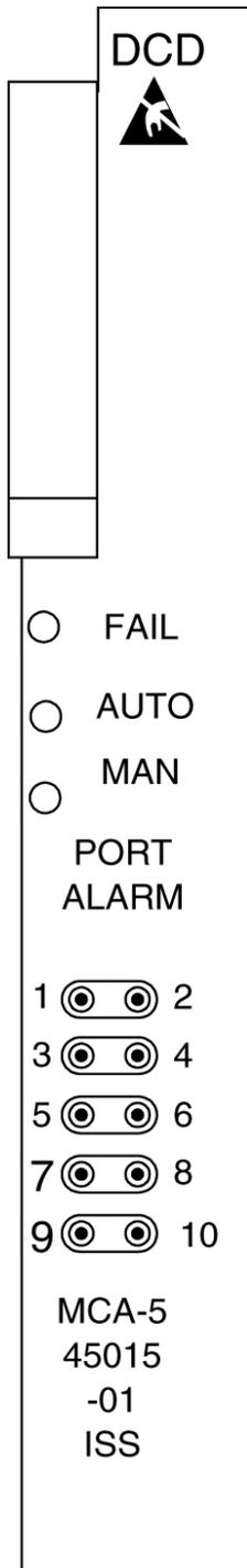
Figure 151: Holdover Clock MCA Card LEDs
