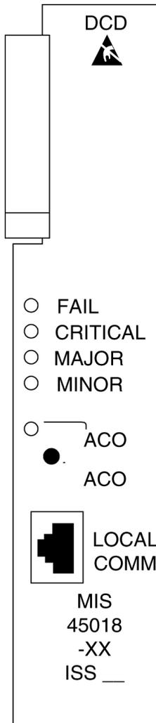
Figure 150: Holdover Clock MIS Card LEDs
