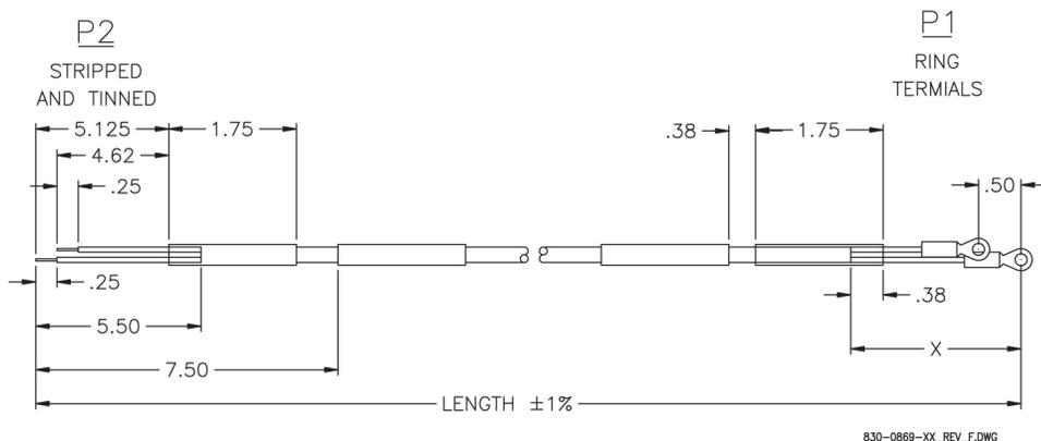
Figure 248: Router Power Cable
