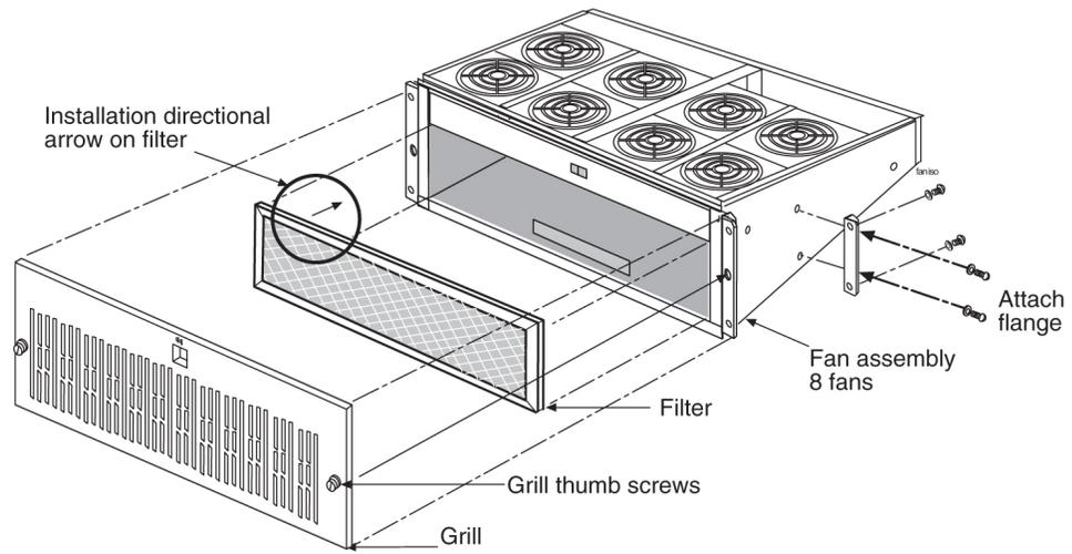
**Figure 93: Fan Assembly with Grill and Filter**
