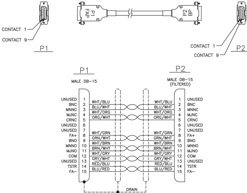
Figure 220: Filter Rack Alarm Cable
