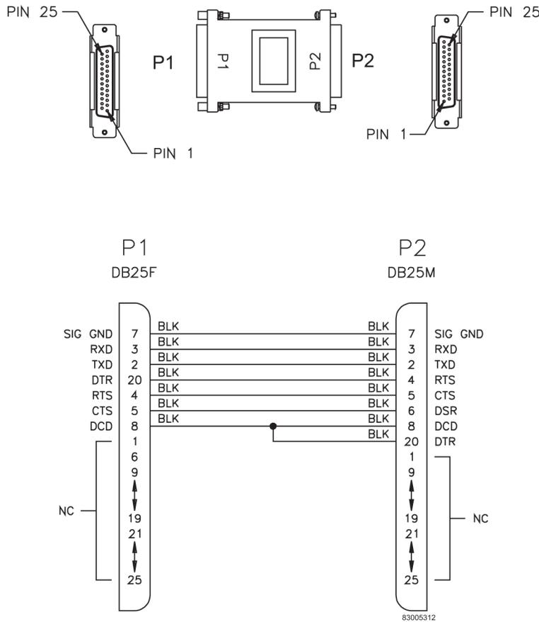
Figure 252: Serial Interface, Adapter
