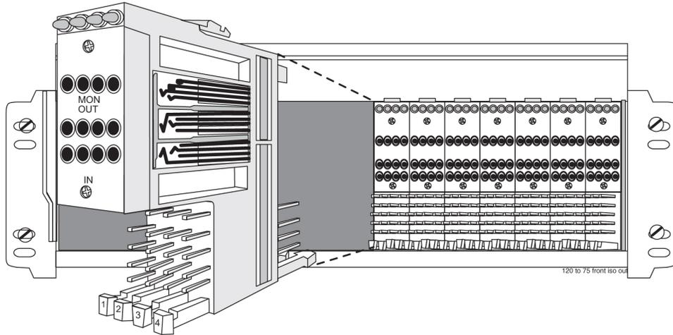
Figure 130: 120 Ohms Converter and Shelf
