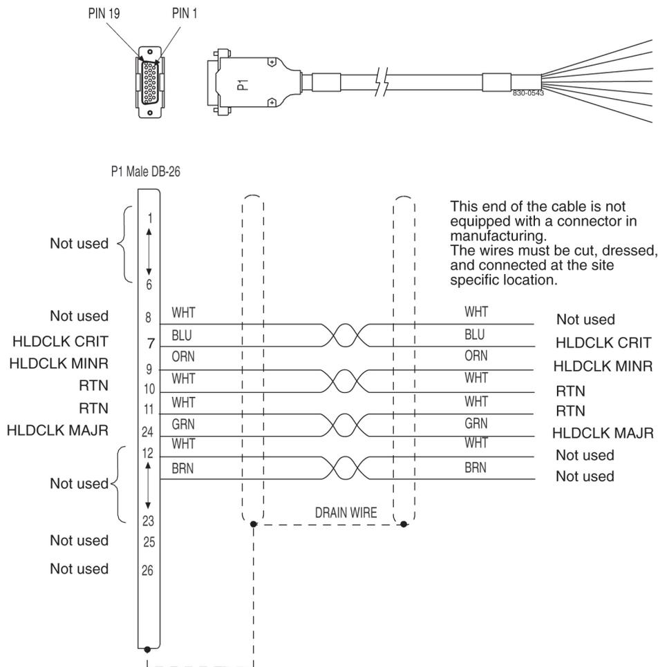
**Figure 198: Holdover Clock Alarm Cable**
