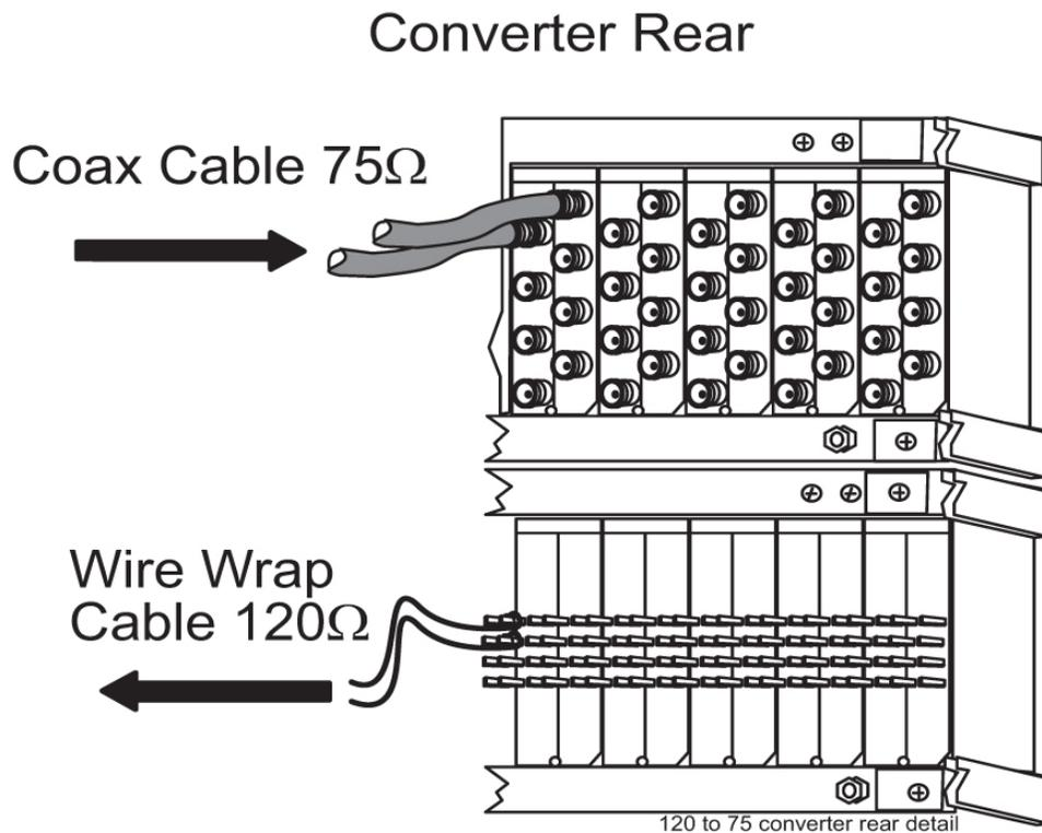
Figure 133: Converter Rear Detail
