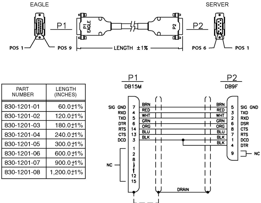
Figure 257: Terminal Server Serial Cable with Flow Control (P/N 830-1201-xx)
