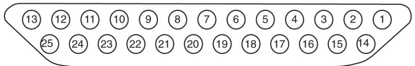
Figure 172: Clock B In Connector on Backplane
