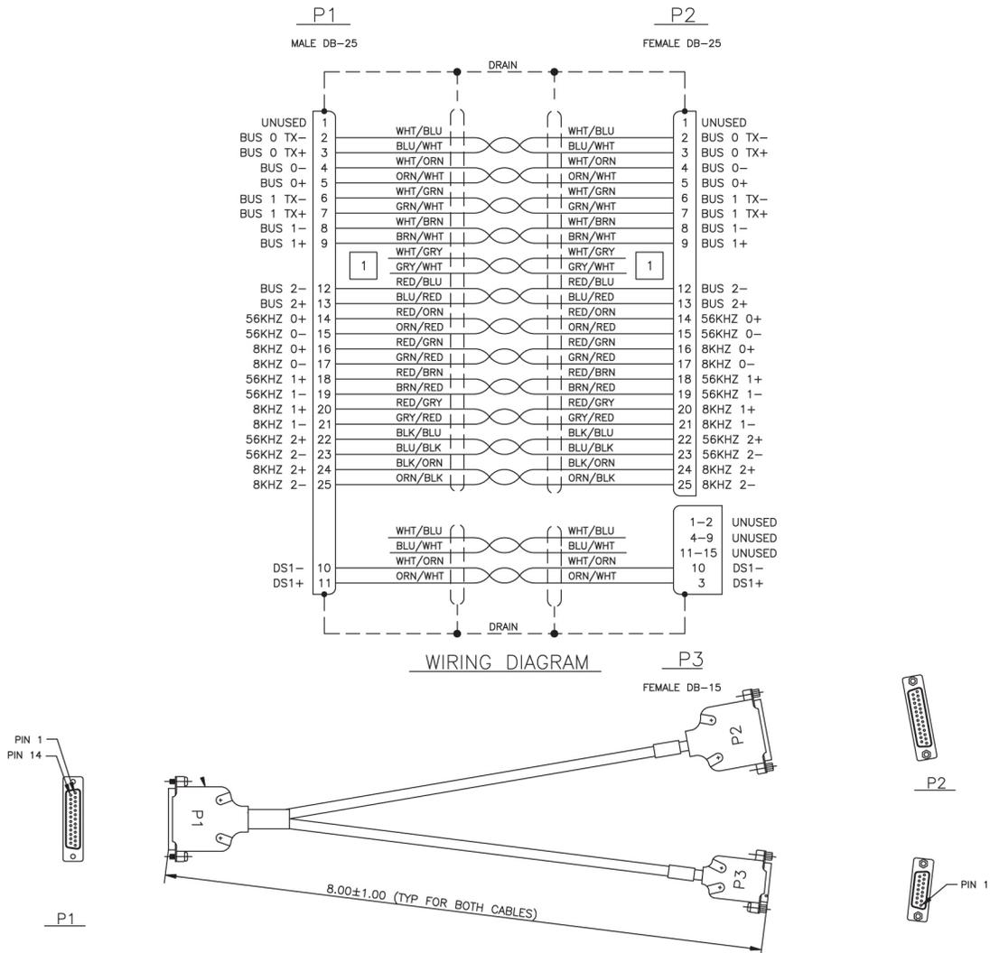
Figure 223: High Speed Master Timing Adapter
