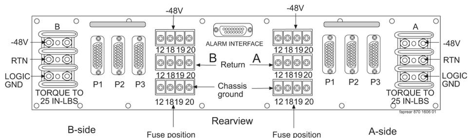
**Figure 56: 3U Fuse and Alarm Panel Rear (P/N 870-2320-03)**
