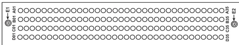
Figure 177: Control Shelf Backplane Pin-Outs, Top Connector
