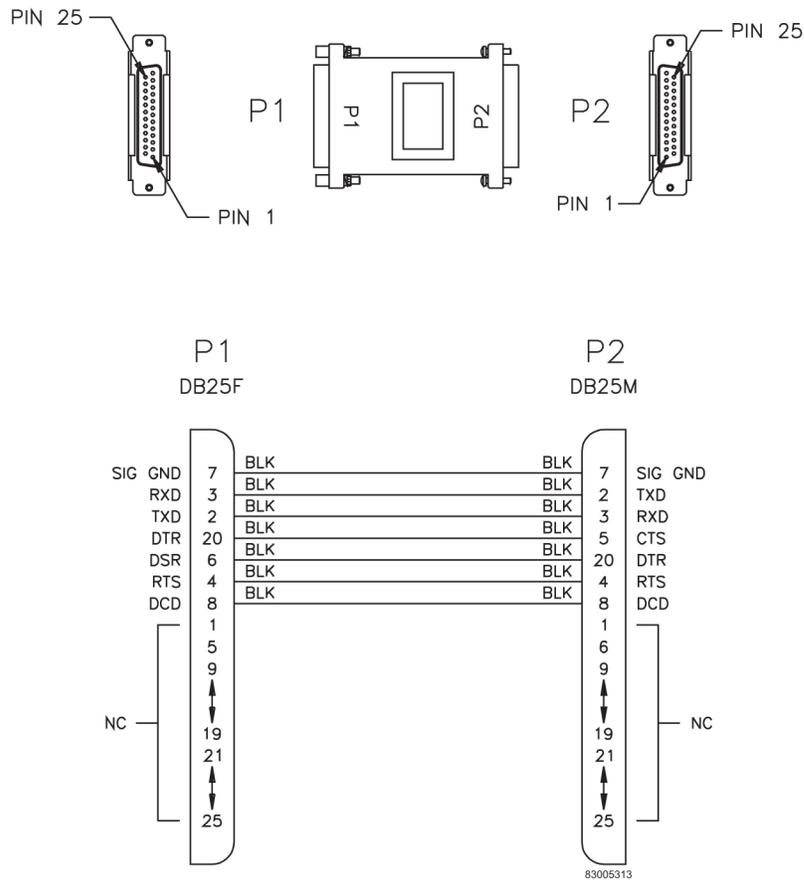
**Figure 251: Serial Interface/Modem Adapter**
