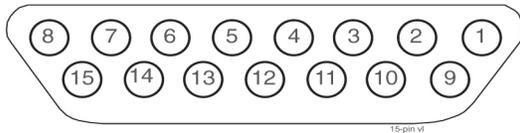
Figure 174: BITS Clock Connector
