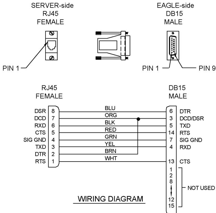
Figure 260: Terminal/Server Serial Port Adapter, EAGLE/Cyclades (P/N 830-0915-03)
