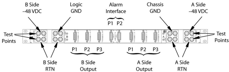
**Figure 55: 1U Fuse and Alarm Panel Rear (P/N 870-2804-01)**
