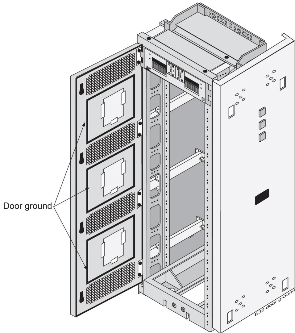
**Figure 27: EAGLE 5 ISS Frame with Door Ground**
