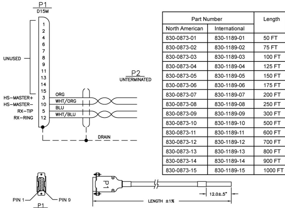
Figure 229: Master Clock Cable (BITS/High-speed)
