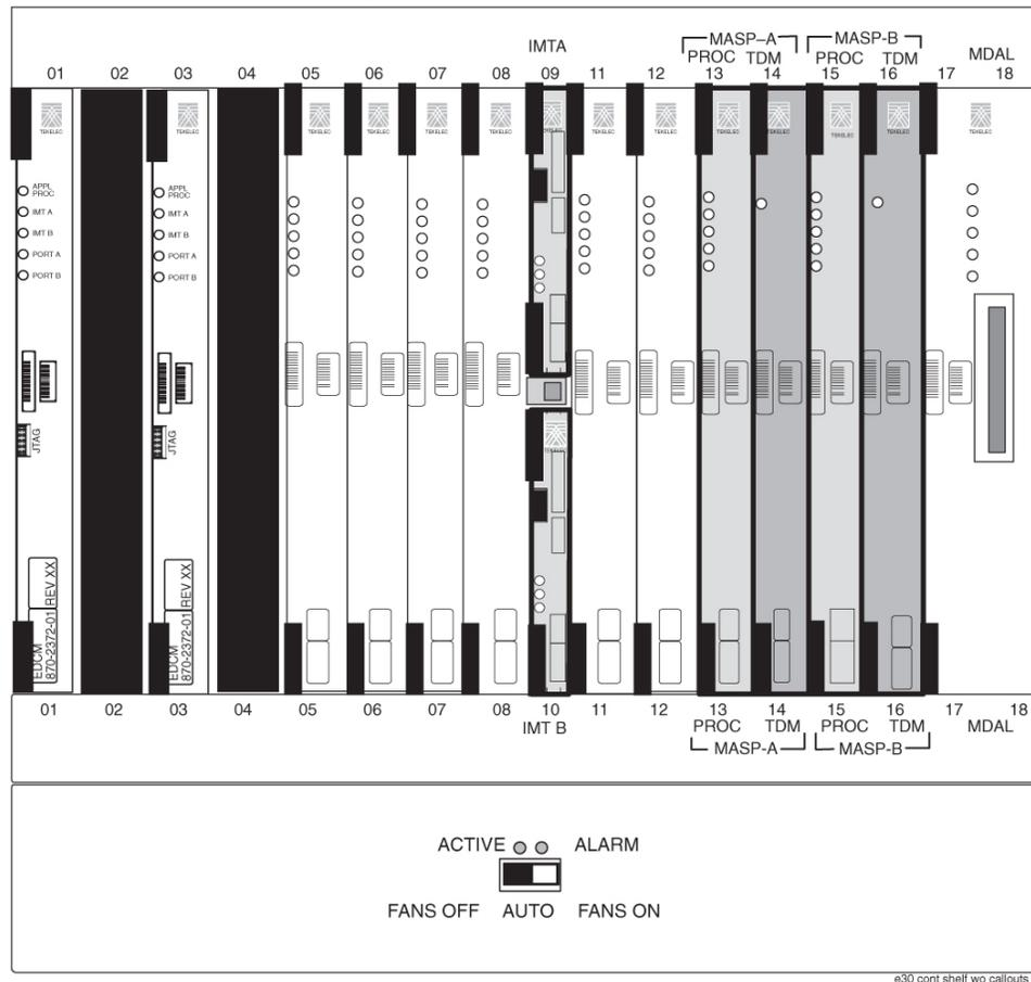
**Figure 97: Front Card Suite with Fan Switch**
