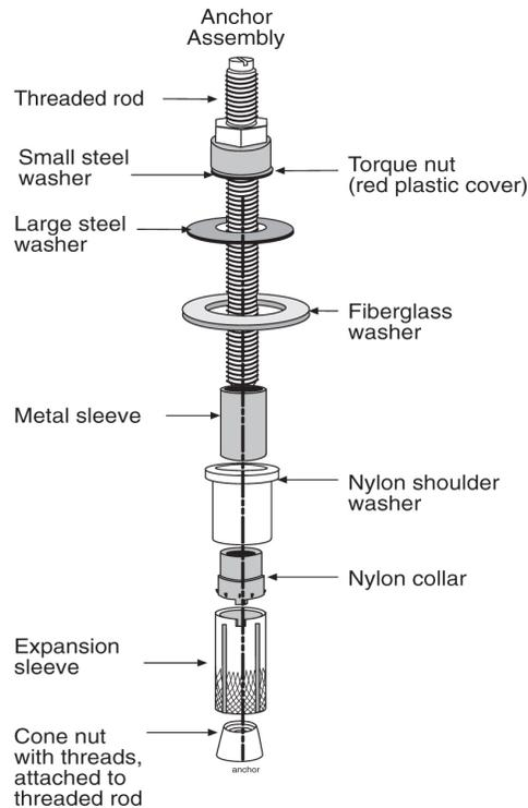
**Figure 21: Anchor Assembly**
