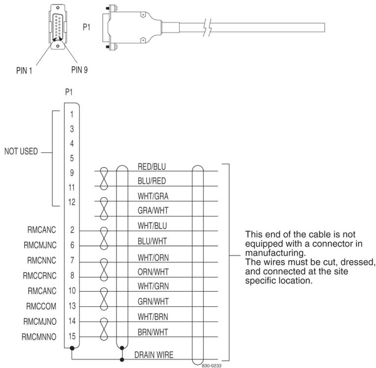
Figure 243: Remote Maintenance Center Cable
