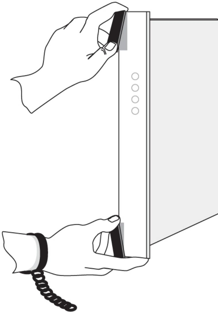
**Figure 5: Removing an EAGLE 5 ISS card**
