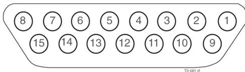
**Figure 163: Remote Maintenance Center Alarm Connector**
