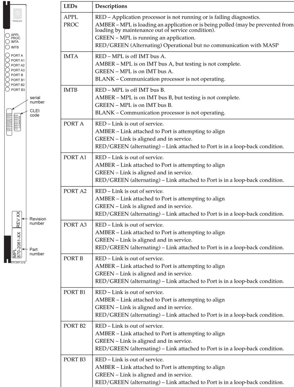
Figure 152: MPL LEDs
