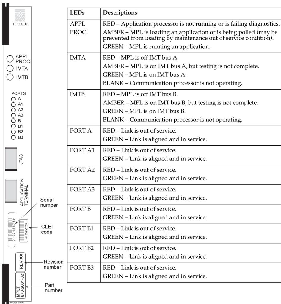
Figure 153: MPLT LEDs
