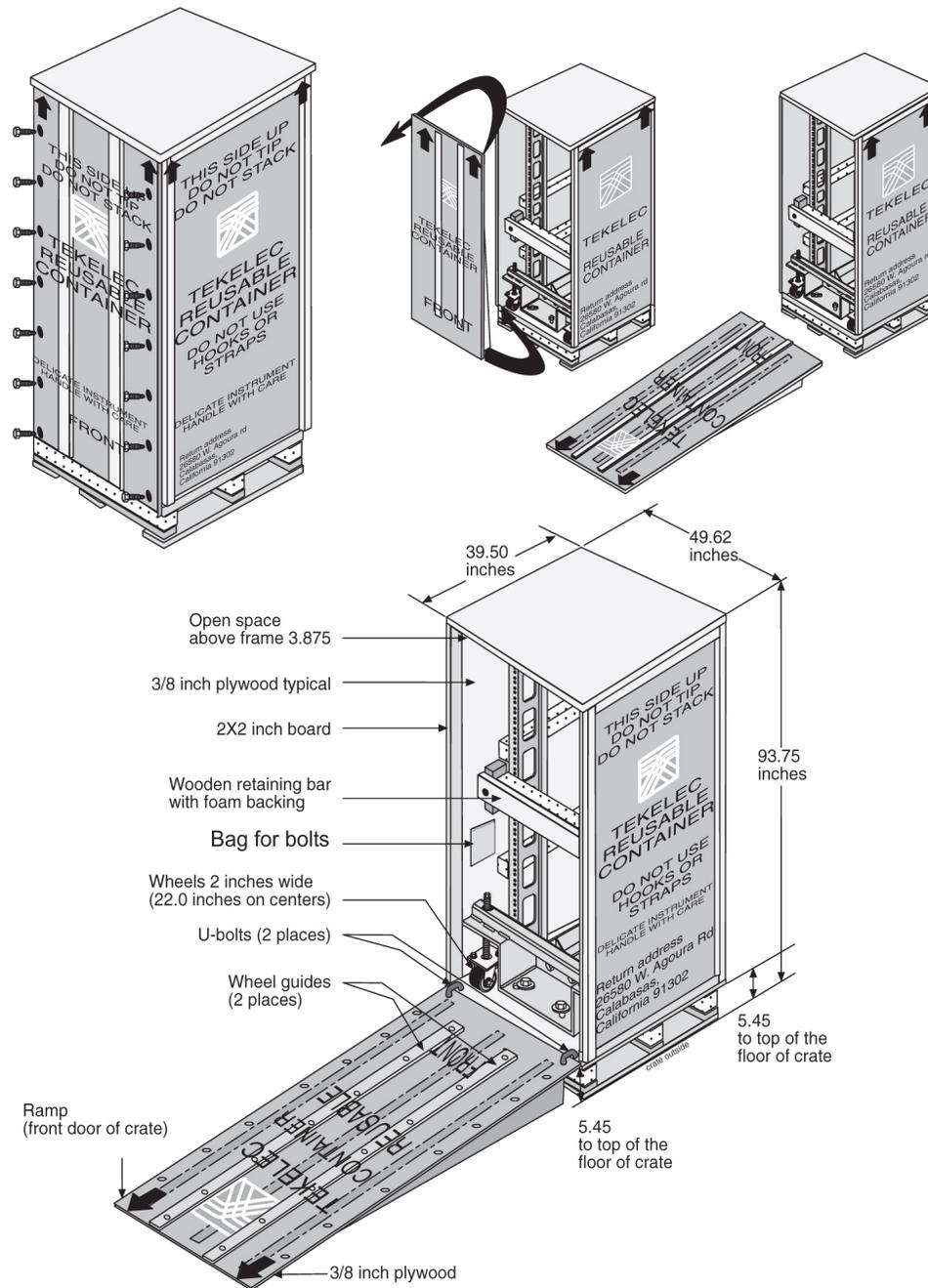
**Figure 10: Shipping Container for Heavy Duty Frame**
