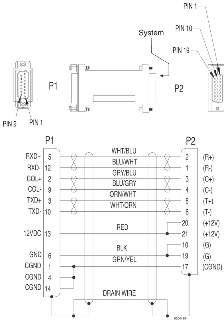
**Figure 217: ENET Adapter 15-Pin to 26-Pin (P/N 830-0425-01)**
