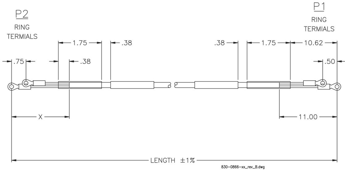
Figure 203: Power Cable to Breaker Strip
