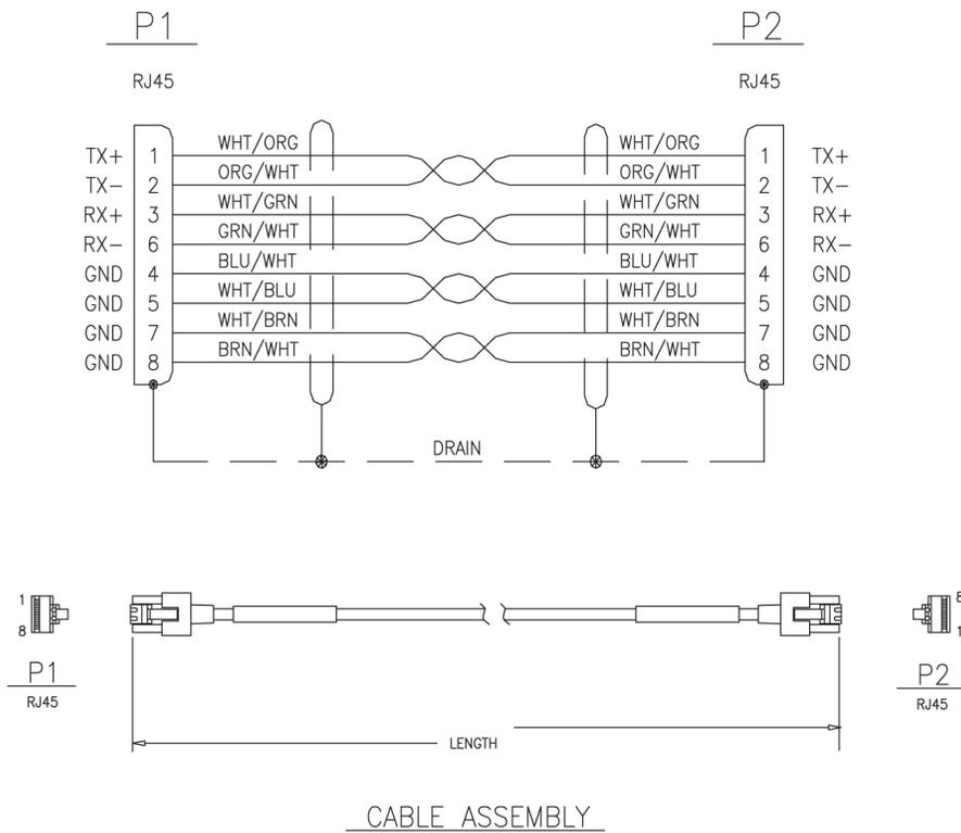
Figure 245: RJ45/RJ45 Cable (CAT-5)
