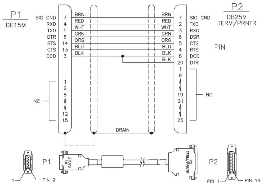
Figure 231: Man-Machine Interface Port Cable
