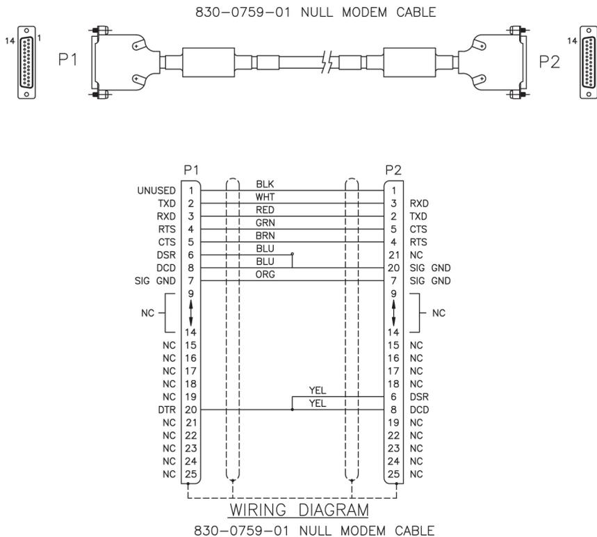
Figure 238: Null Modem Cable
