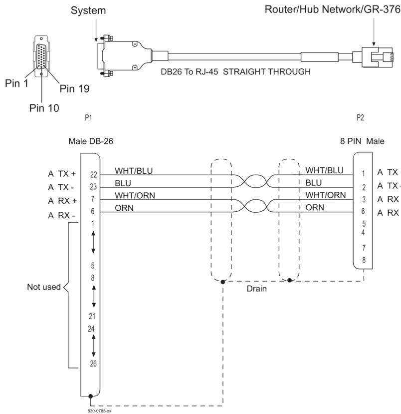
Figure 254: Straight Through Patch Panel Cable
