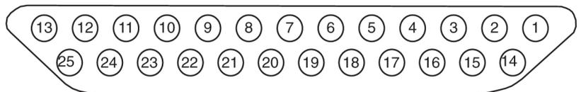
Figure 185: General Purpose Relay Connector 02
