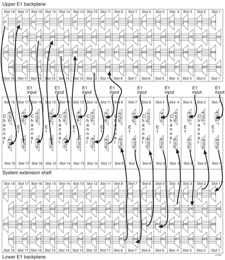
Figure 126: E1 Interface Backplane Connections
