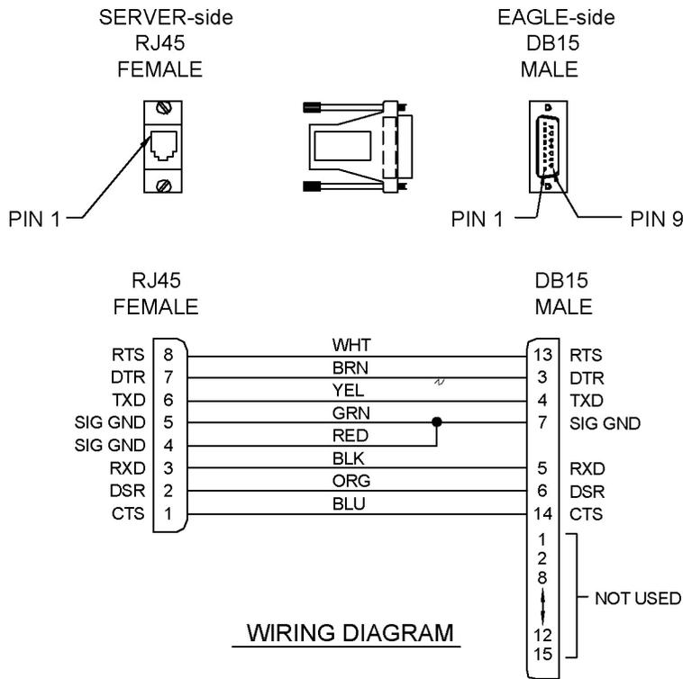
Figure 258: Terminal/Server Serial Port Adapter, NTW (P/N 830-0915-01)
