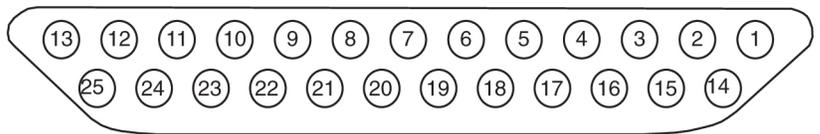
**Figure 192: Clock B Out Extension Shelf Connector**
