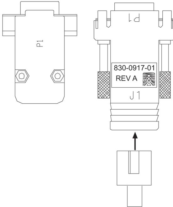
Figure 246: RJ 45 to 9 Pin Adapter
