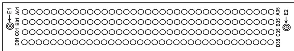
**Figure 194: Extension Shelf Backplane Pin-Outs, Top Connector**
