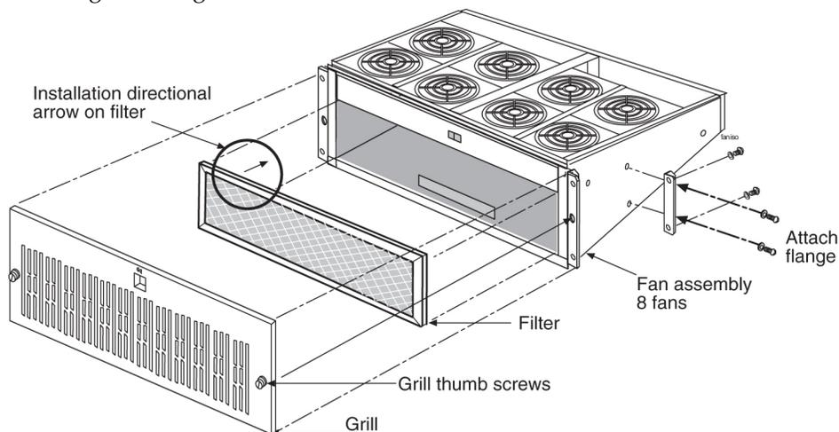
**Figure 98: Fan Assembly with Grill and Filter**
