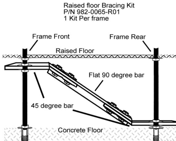
**Figure 20: Earthquake Bracing**
