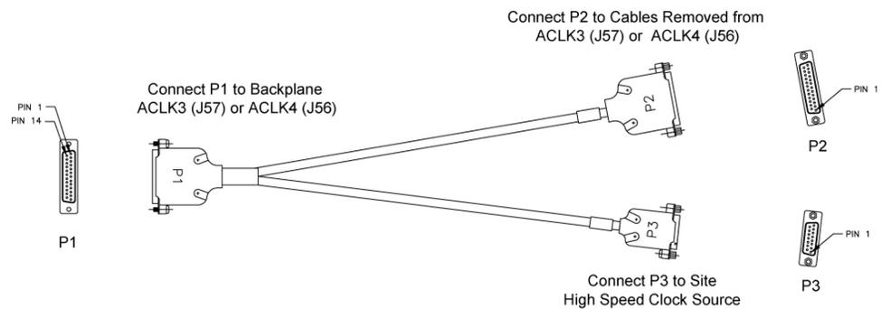
**Figure 104: High-Speed Master Timing Adapter Cable (P/N 830-0846-01)**
