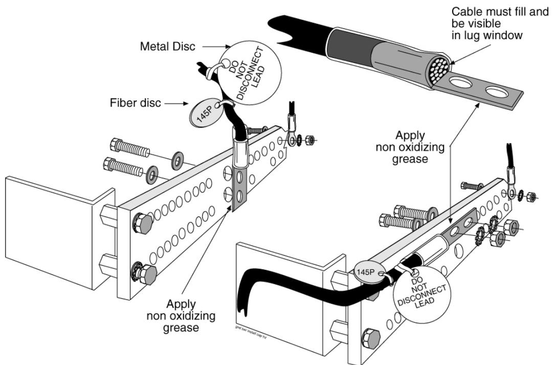
**Figure 57: Ground Bar and Logic Ground Installation**
