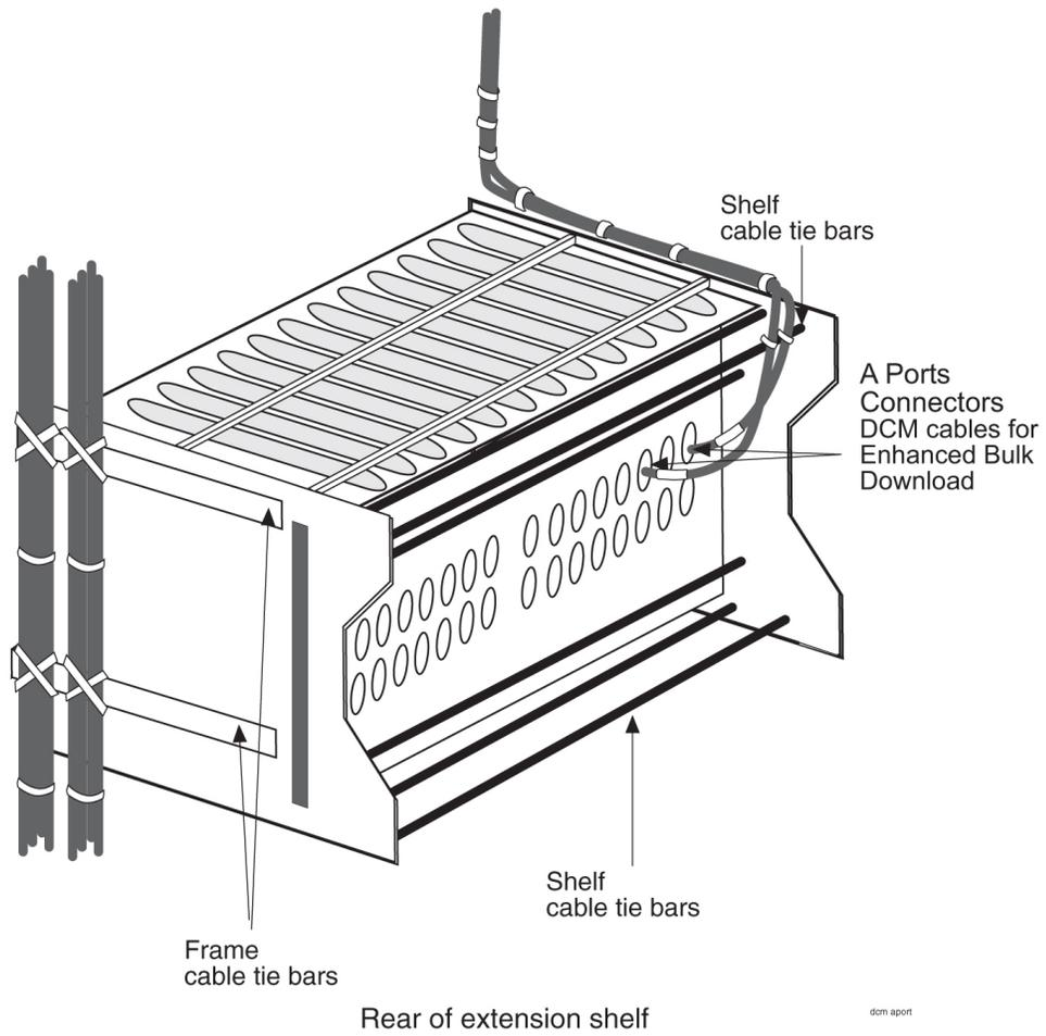
**Figure 76: DCM Family Cabling, Enhanced Bulk Download**
