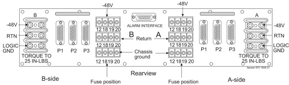
**Figure 157: Control/Extension FAP Rear View**
