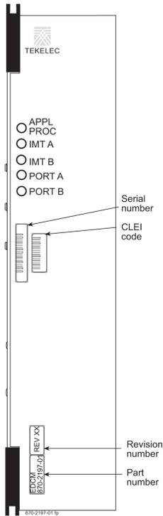
Figure 146: EDCM (Double-Slot) LEDs
