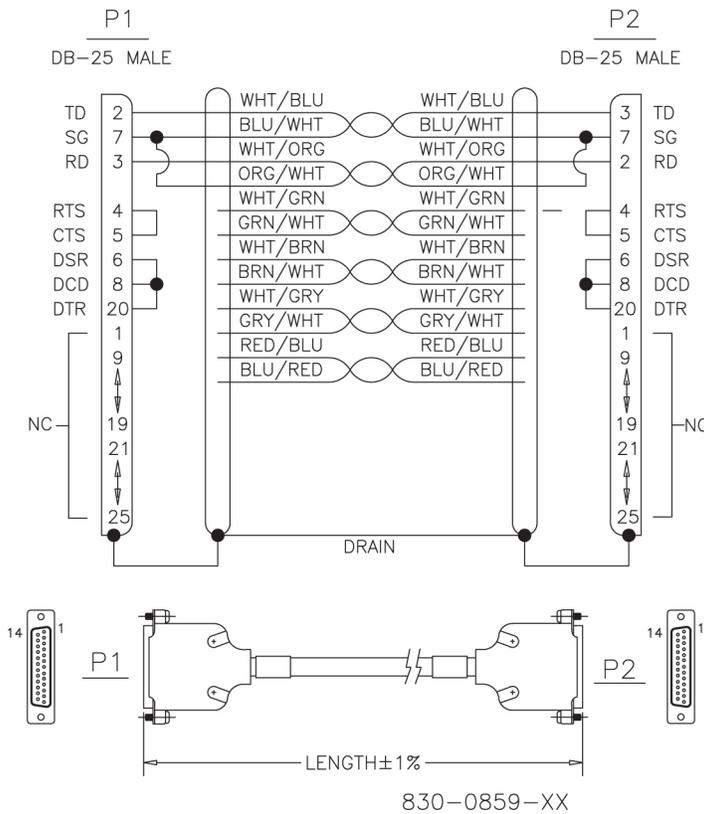
Figure 239: Null-MODEM for Terminal
