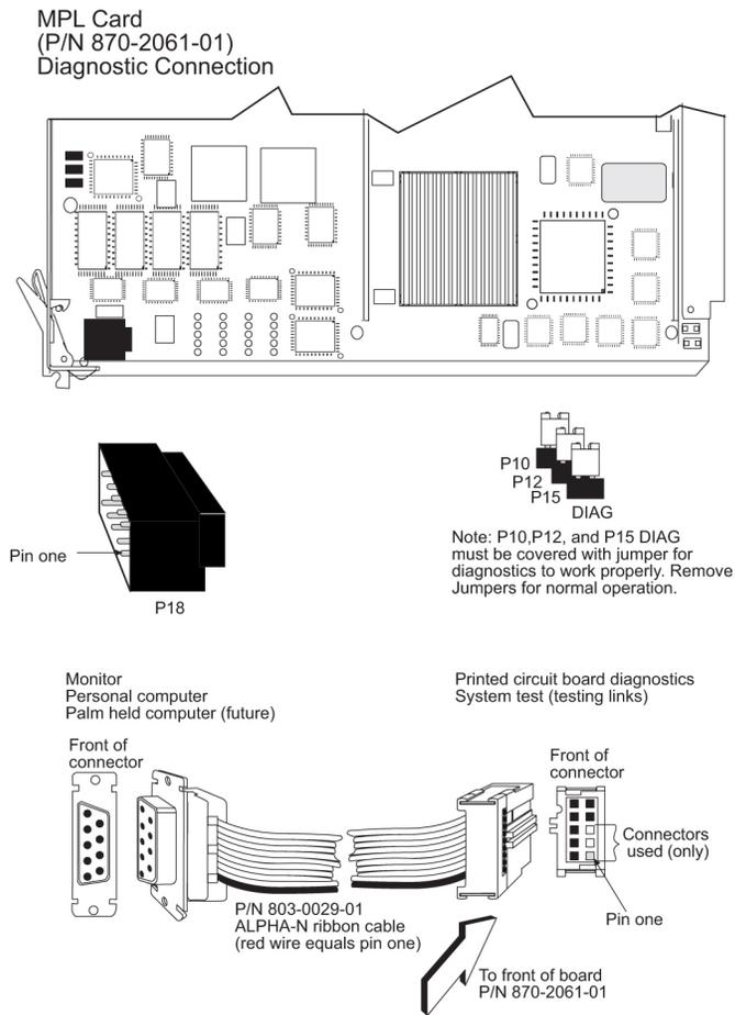
Figure 233: MPL Card Diagnostic Cable
