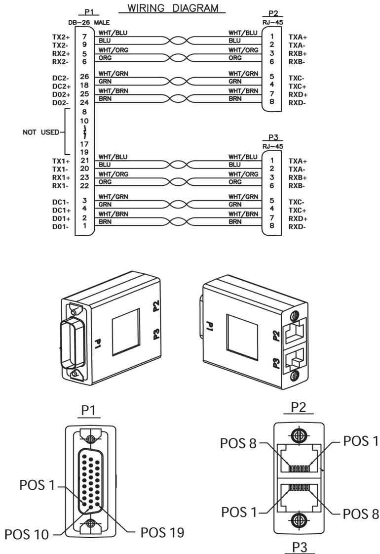
Figure 213: DB26 Male to Dual RJ45 Adapter
