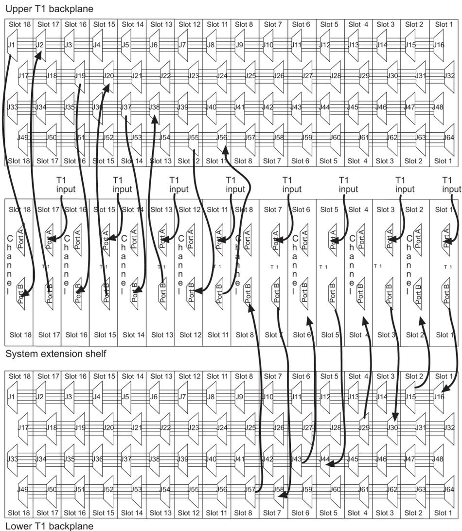
Figure 127: T1 Interface Backplane Connections
