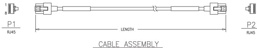
Figure 244: RJ45/RJ45 Cable (CAT-5)
