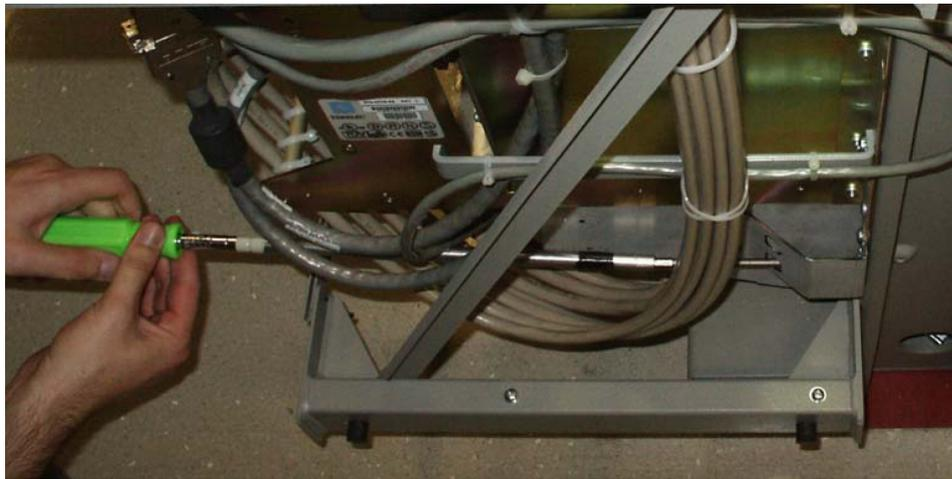
**Figure 90: Tighten fan side bracket screws**
