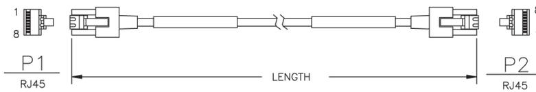
Figure 253: Straight Through Cable (CAT-5)
