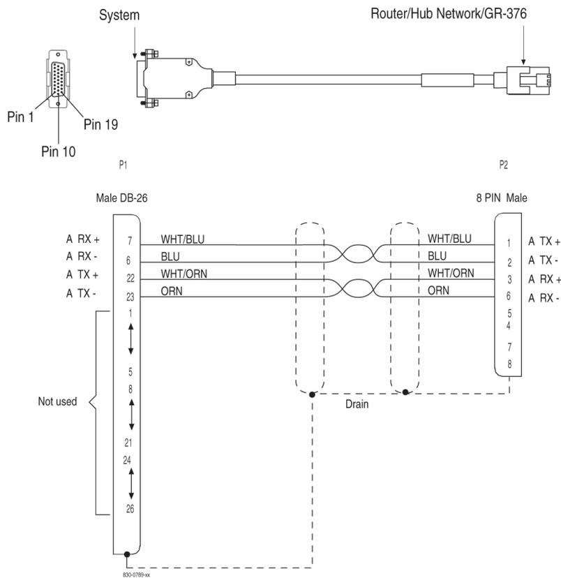
Figure 206: Crossover DCM Patch Panel Cable
