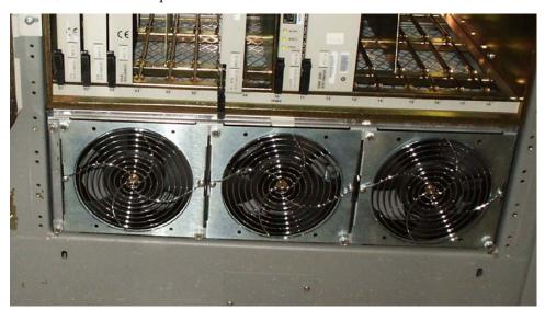
Figure 88: Fan tray inserted into fan tray bracket in the frame- front view
