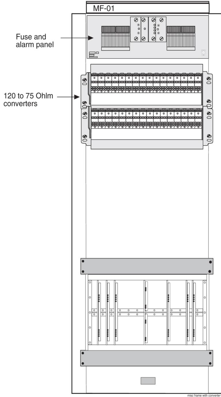
Figure 129: Miscellaneous Frame with 120 Ohm Converter
