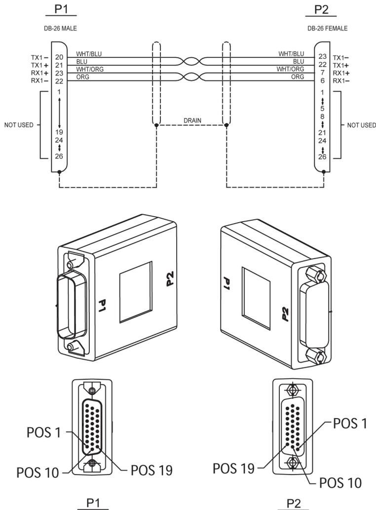
Figure 214: DB26 Male-to-DB26 Female Adapter
