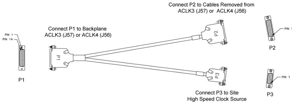
Figure 230: Master High Speed Clock Adapter
