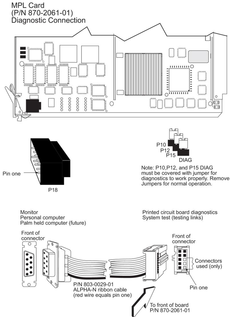
Figure 128: MPL Card Diagnostic Cable
