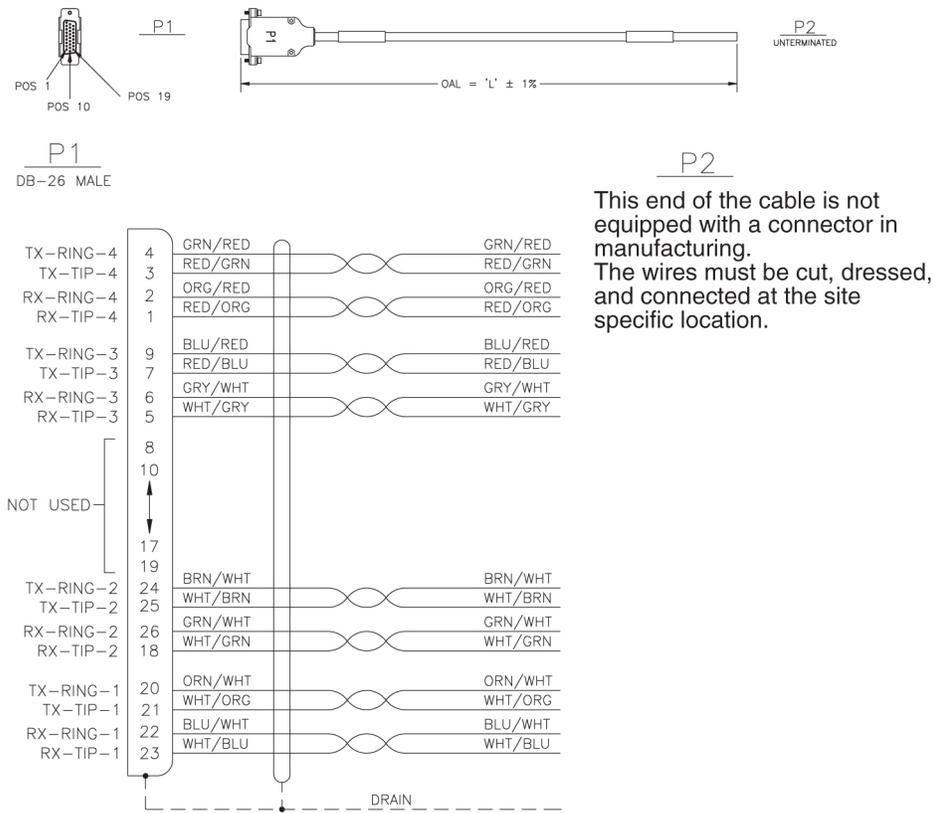
This end of the cable is not equipped with a connector in manufacturing. The wires must be cut, dressed, and connected at the site specific location.
