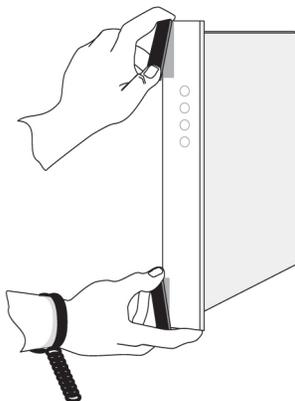
**Figure 120: Removing a Card**
