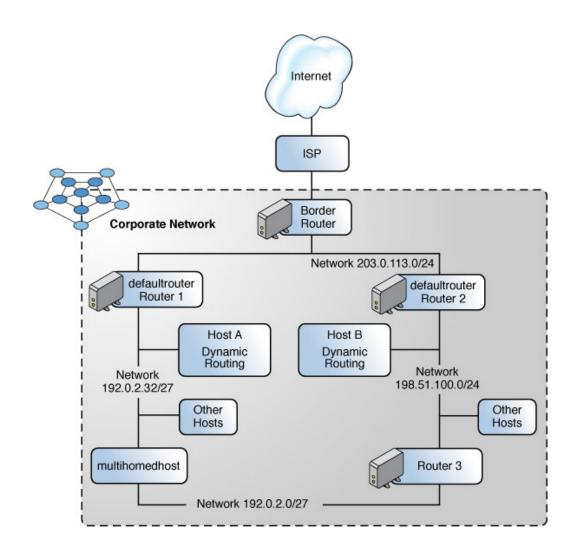
Router 2 contains two wired network connections, one connection to network 198.51.100.0 and one to network 203.0.113.0. The example shows how to configure a system as a router (Router 2) of the 198.51.100.0 network. The example also assumes that Router 2 has been configured to operate in the local files mode as described in "How to Configure a System for Local Files Mode" in *Configuring and Managing Network Components in Oracle Solaris 11.3*.
