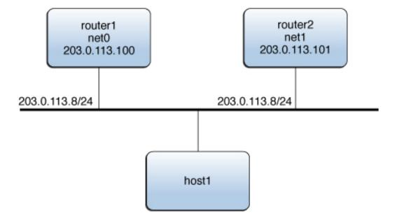
In this example, the IP address 203.0.113.8 is configured as the default gateway for host1. This IP address is the virtual IP address that is protected by the virtual router that consists of two VRRP routers: router1 and router2. At any given time, only one of the two routers serves as the master router, assuming the responsibilities of the virtual router and forwarding packets that come from host1.
