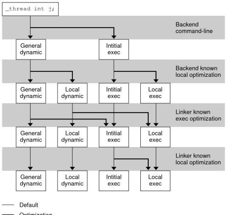
FIGURE 19 Thread-Local Storage Access Models and Transitions
