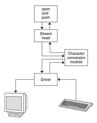
FIGURE 9 Pushing the Character Conversion Module
