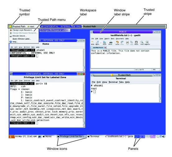
FIGURE 6 Trusted Extensions Multilevel Desktop
