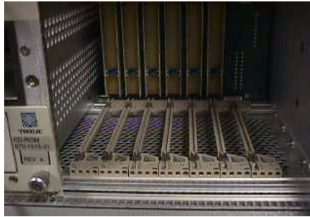
Figure 6-50. EOAP Backplane Connector Pins
