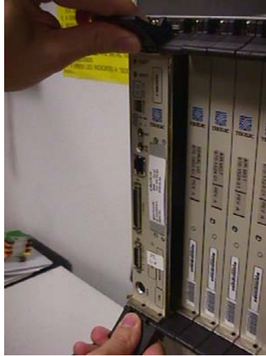
Figure 6-62. Inserting the Replacement Processor Card
