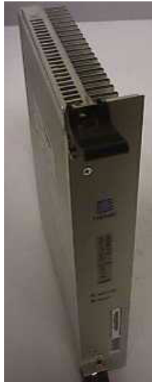
Figure 6-51. Power Supply Card (P/N 870-1521-01)
