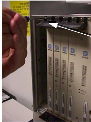
Figure 6-67. Top Handle and Captive Screw of Serial Card
