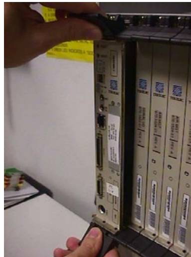
Figure 3-41. Inserting the Card
