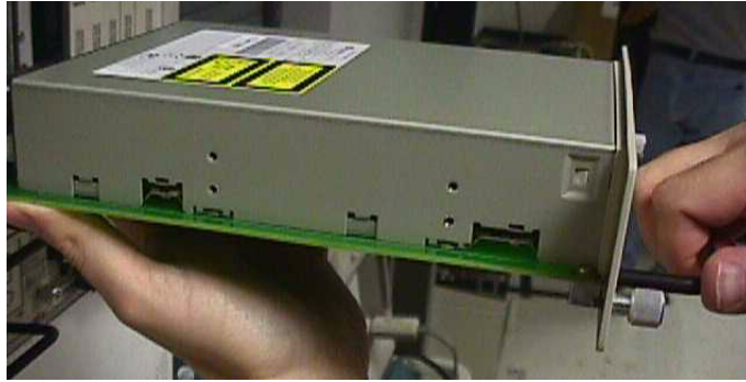
Figure 6-27. Support the CD-ROM Drive Card With Both Hands
