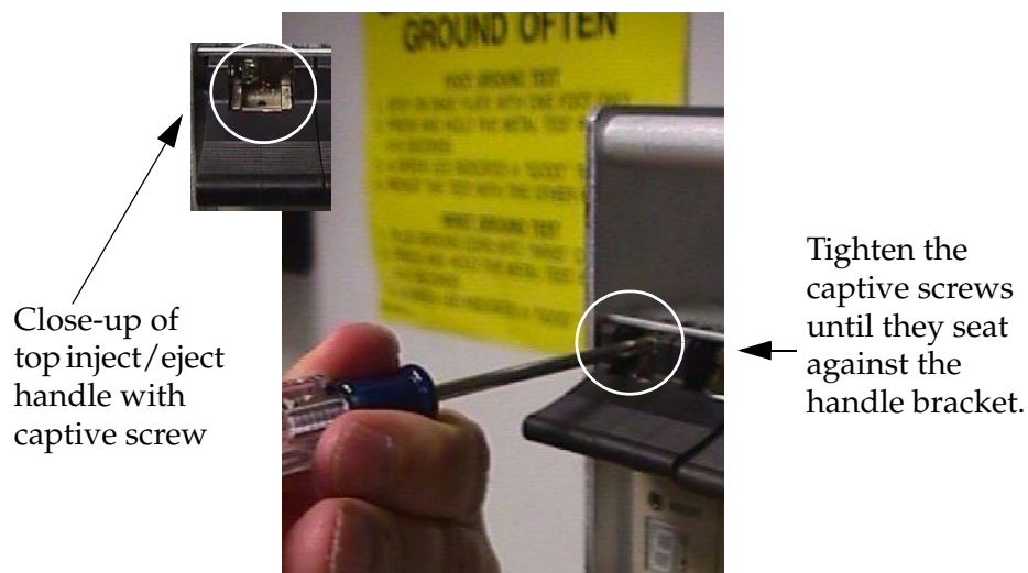
Figure 6-64. Tightening Captive Screws
