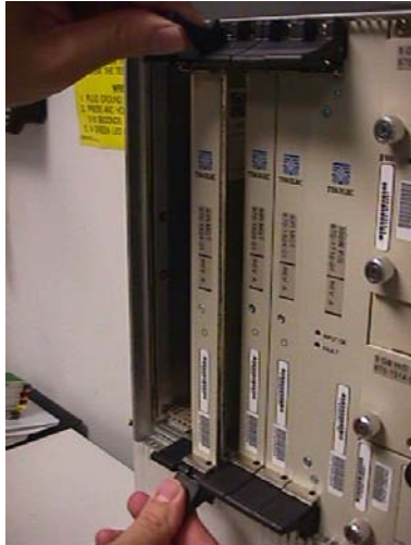
Figure 6-5. Inserting the Replacement Air Management Card
