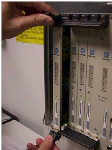
Figure 6-72. Inserting the Replacement Serial Card
