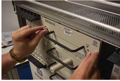
Figure 6-40. Loosen Hard Drive Card Captive Screws
