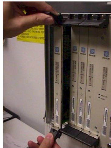
Figure 6-68. Freeing the Card from the EOAP Card Cage
