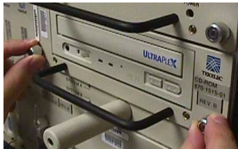
Figure 6-26. CD-ROM Drive Card Captive Screws
