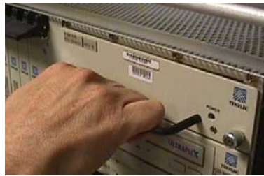
Figure 6-41. Free Hard Drive Card from the EOAP Card Cage
