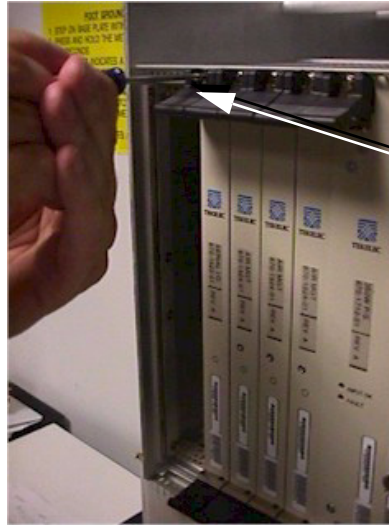
Figure 6-74. Tighten Captive Screws
