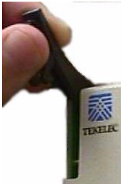
Figure 3-7. Push Inject/Eject Clamps Outward
