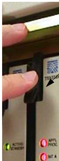
Figure A-18. Push in Inject/Eject Clamps
