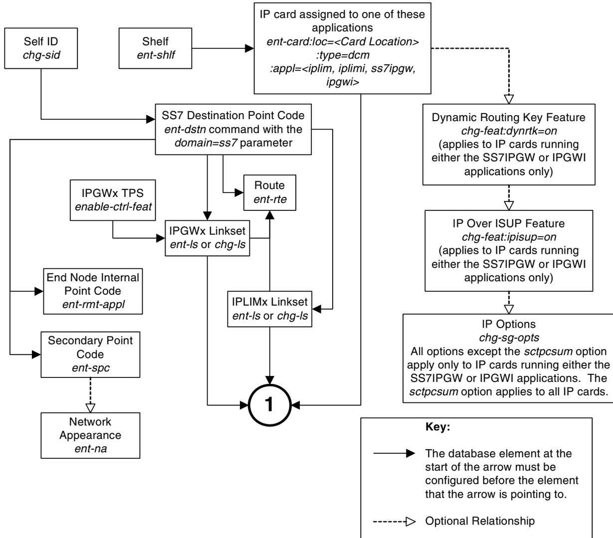
Figure 3-2. IP<sup>7</sup> Secure Gateway Database Relationships (Sheet 2 of 2)
