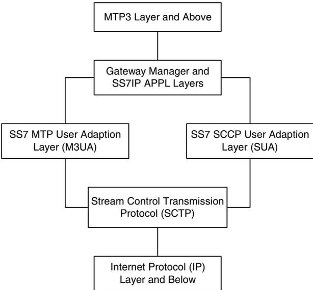
The EAGLE 5 ISS supports many (mapping & transport) protocol combinations. One connection can be running TALI/TCP while another connection is running M3UA/SCTP, and a third connection is running M2PA/SCTP. These three connections can be on the same card (provided the card is an IPGWx card) and even a part of the same routing key (if the card is an IPGWx card). If the card is an IPLIMx card, only M2PA connections can be assigned to the card.
