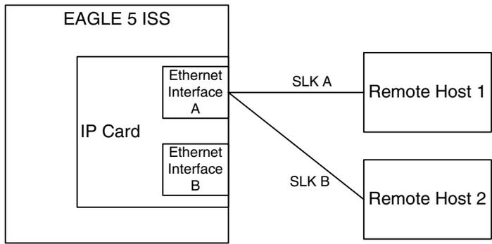
**IP Connection on a Dual-Slot DCM Running the IPGWx Application**
