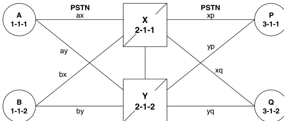
**Figure 5-7.** Network after Two Signaling End Points Migrate from PSTN to IP
