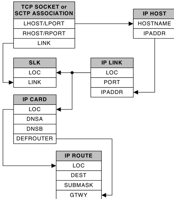
There is no direct correlation between signaling link ports and Ethernet interfaces. A card can be using Ethernet interface A and signaling link B to transmit data to the remote host. Another scenario could have the card using Ethernet interface B and signaling link A to transmit data to the remote host.
