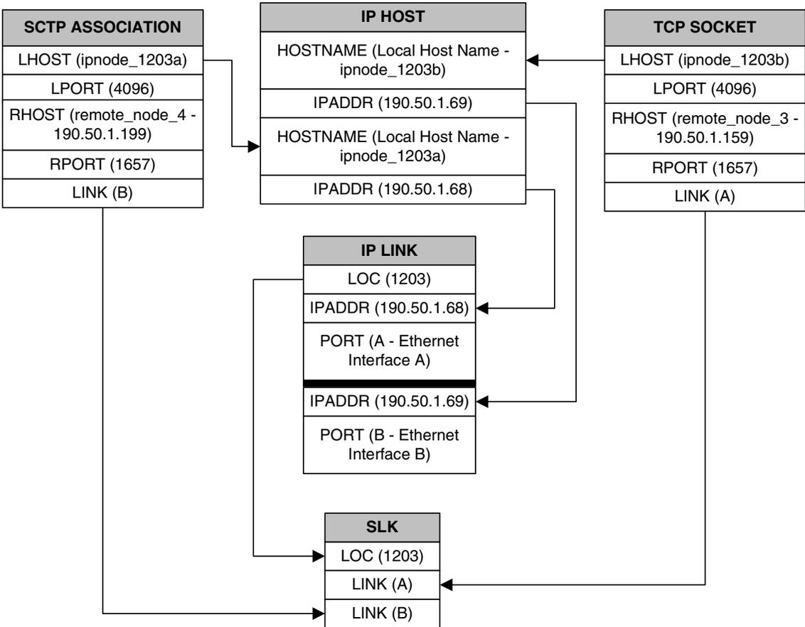
**IP Connection on a Single-slot EDCM Running the IPLIMx Application**
