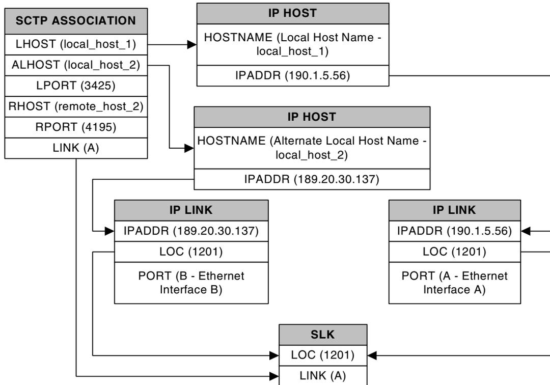
Using the data shown in Figure 2-11, the IP connection is defined as a multi-homed association, connecting to a remote host using local hosts 190.1.5.56 and 189.20.30.137 over Sctp port 3425, using signaling link B on card 1201.
