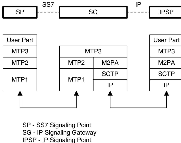
The M2PA layer receives the primitives sent from MTP3 to its lower layer. The M2PA layer processes these primitives or maps them to appropriate primitives at the M2PA/SCTP interface. Likewise, the M2PA layer sends primitives to MTP3 like those used in the MTP3/MTP2 interface.
