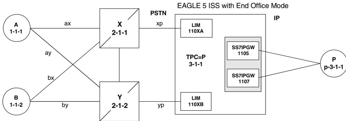
In Figure 5-3 the EAGLE 5 ISS no longer acts like a signaling transfer point, but rather acts like a signaling end point that has an IP-attached application user-part. The EAGLE 5 ISS and the IP network element share the point code P. All messages received by the EAGLE 5 ISS should be destined to P and all messages sent to the PSTN from the EAGLE 5 ISS have an OPC of P.
