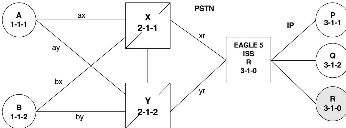
In Figure 5-5 the customer saves a point code by using the End Office feature and making the new IP network element an end office node. No change is required in the PSTN or at P or Q. Non-network-management and non-test messages destined to R are now forwarded to an IP network element, rather than terminated by the EAGLE 5 ISS.
