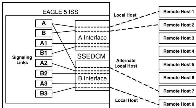
**IP Connection on an E5-ENET Card Running the IPLIMx Application**
