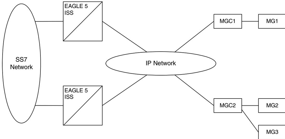
The EAGLE 5 ISS maps the originating point code, destination point code, and circuit identification code to an IP connection. The SEP is provided the originating and destination point codes in the MTP level 3 routing label as part of the passed protocol.
