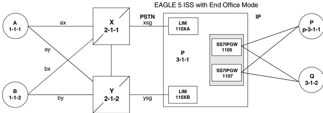
In Figure 5-7, P is an end office node, and so P serves as the adjacent point code for nodes X and Y. The following are key points about this figure:
