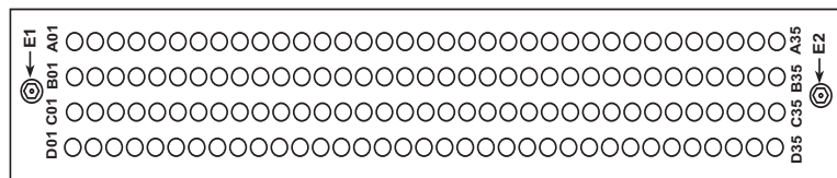
Figure B-20. Extension Shelf Backplane Pin-Outs, Bottom Connector
