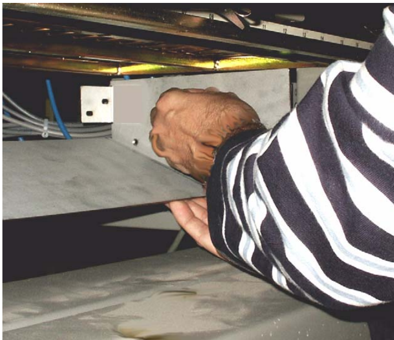
Figure 5-18. Attaching the fan tray bracket to the side brackets - inside front
