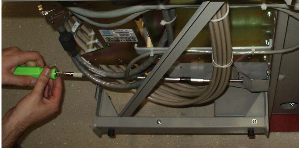
Figure 5-22. Tighten fan side bracket screws
