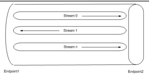
The multiple stream mechanism is designed to solve the head-of-the-line blocking problem of TCP. Therefore, messages from different multiplexed flows do not block one another.
