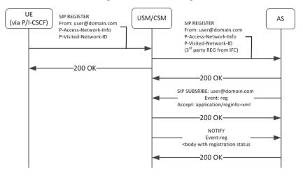
This feature is relevant when the Oracle USM is performing S-CSCF functions. You enable this feature on the Oracle USM per registrar, by simply creating a profile and applying it to the applicable registrar.
