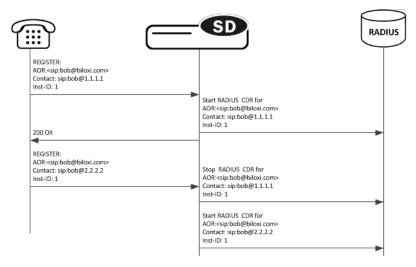
Similarly, when the Oracle USM receives a REGISTER for an existing Contact and AoR but with a different Instance-ID, the registration is updated by the Oracle USM. The same corresponding stop and start CDRs are sent to the RADIUS server.
