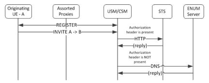
If the STS returns a 200 OK, the Oracle USM proceeds with authentication. If the STS does not reply or is not reachable, the Oracle USM replies to the UA with a 500 Internal server error. If the STS replies with any message other than a 200 OK, the Oracle USM replies to the UA with a 403 Forbidden.
