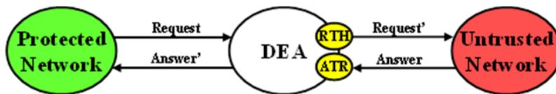
**Figure 3: Diameter Topology Hiding Trigger Points: Protected-to-Untrusted Transactions**
