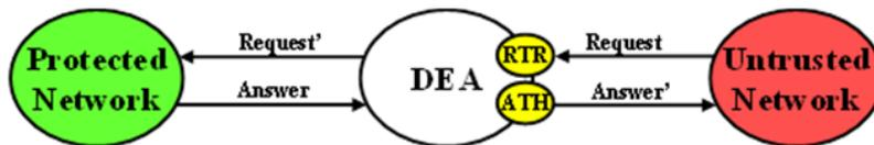
**Figure 4: Diameter Topology Hiding Trigger Points: Untrusted-to-Protected Transactions**
