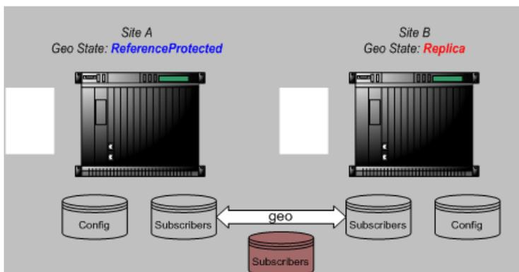
Figure 62: Final State Of The Geo-redundant Sites After Restoring The 'Subscribers' Database Backup
