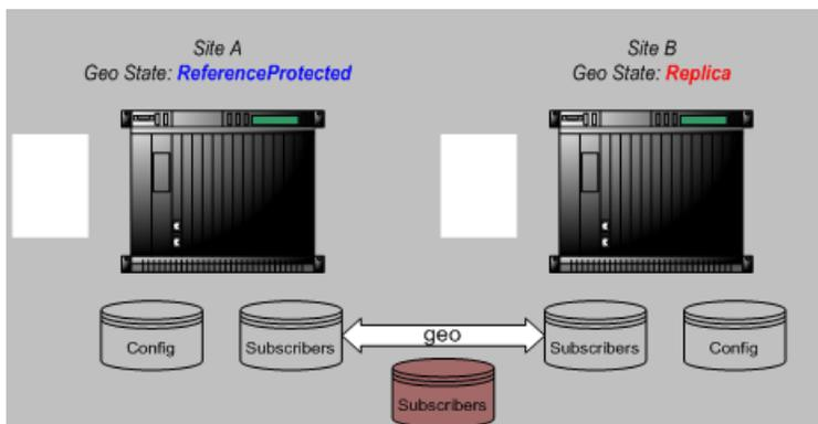
Figure 64: Final State After Restoring A Full Backup On The Reference Site
