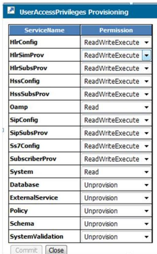
Figure 11: UserAccessPrivileges provisioning window
