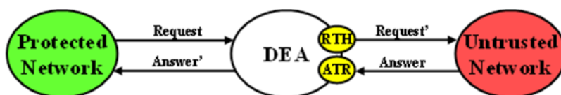
Figure 3: Diameter Topology Hiding Trigger Points: Protected-to-Untrusted Transactions
