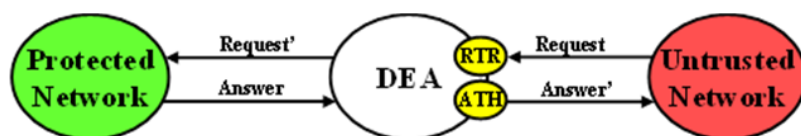
Figure 4: Diameter Topology Hiding Trigger Points: Untrusted-to-Protected Transactions
