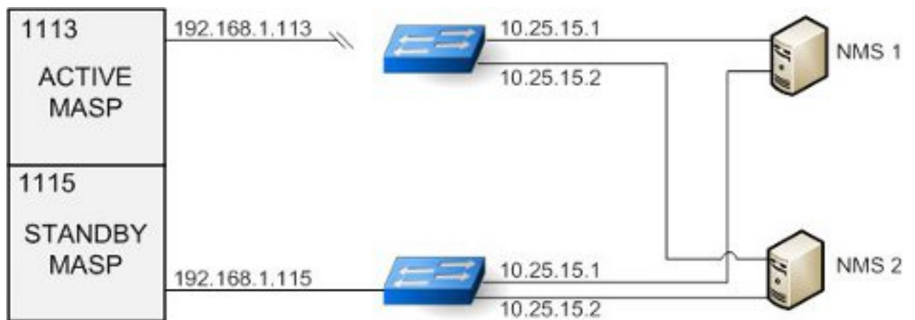
Figure 7: UAM/UIM Trap Flow with Active Link Down
