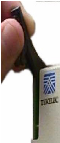
Figure 79: Push Inject/Eject Clamps Outward
