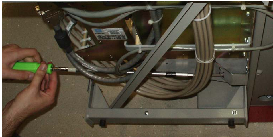
Figure 90: Tighten fan side bracket screws
