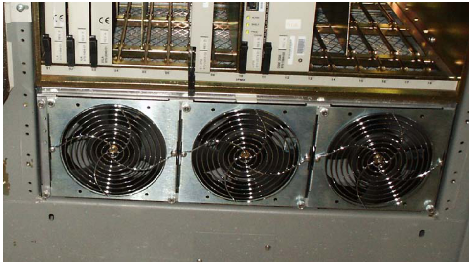
Figure 88: Fan tray inserted into fan tray bracket in the frame- front view
