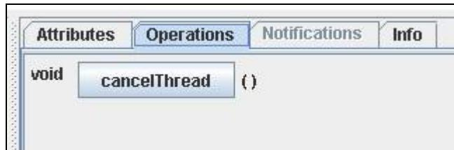
**Note:** Depending on the JMX console used, a confirmation dialog may NOT be displayed and cannot be undone once issued. Ensure that the correct thread for the batch process is selected. To cancel a batch process, ALL threads must be cancelled.
