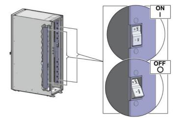
3. Make sure that the circuit breakers located on the rear left and right side power supplies of the Oracle ZFS Storage Appliance ZS3-ES are in the ON (|) position.
