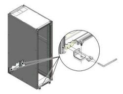
7. Using bolts and washers that are appropriate for your installation site, permanently mount your system to the floor using the four mounting brackets. See Figure 4.8.
