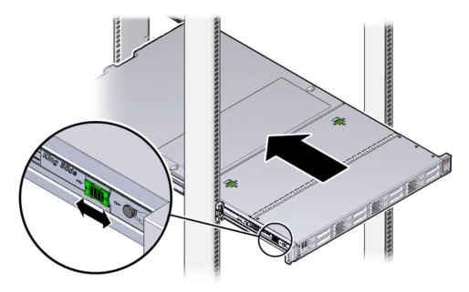
c. Continue pushing the server into the rack until the slide-rail locks (on the front of the server) engage the slide-rail assemblies.
