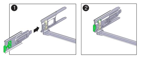
8. While holding the slide-rail latching bracket in place, insert connector D and its associated slide-rail latching bracket into the left slide-rail until connector D locks into place with an audible click. See Figure 6.12, frames 1 and 2.
