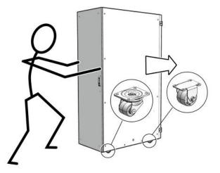
4. When the rack is at the installation site, verify that no components or connections have become dislodged or disconnected during transport. If necessary, re-attach components and cables properly.
