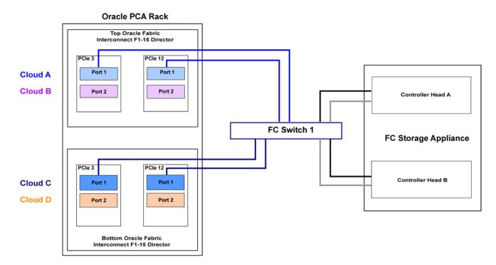
Figure 7.1 Minimum HA FC Storage Cabling Configuration
