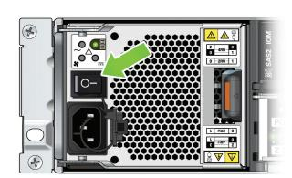
Note: The image shows the circuit breaker on the left power supply. The circuit breaker of the right power supply must also be switched on.
