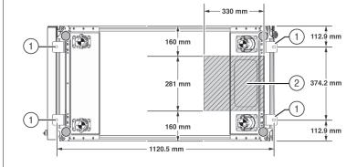
C Optionally, if you plan to route data or power cables through the bottom of the rack, make a rectangular opening (2) in the floor, below the rear portion of the rack, between the two rear casters and behind the RETMA rails.
