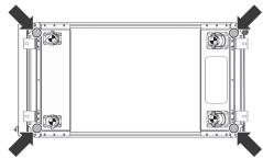
B Lower the leveling feet to the floor using the SW 12mm wrench. The four feet should support the full rack weight.
