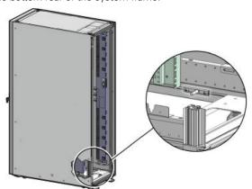
Note: An additional chassis earth ground cable (not supplied) enables electrical current leakage to dissipate more efficiently.
