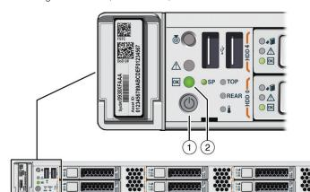
E Wait approximately 5 minutes to allow the management system to power on completely. When complete, the Power/OK LED (2) illuminates and remains a steady green. F On the workstation, browse to the Private Cloud Appliance Dashboard at:
