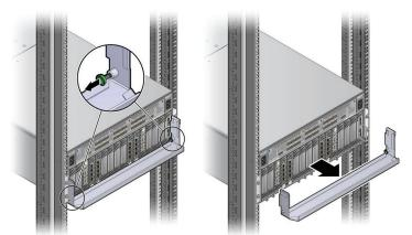
c Carefully pull the bracket away from both Fabric Interconnects, and out
