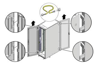
B Remove the filler panel(s) where the expansion node will be installed. The filler panels have snap-in attachments. No screwdriver is required to remove them.
