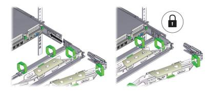
D Align connector C with the slide-rail so that the locking spring is positioned inside (server side) of the right slide-rail.
