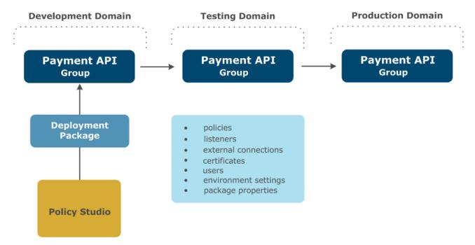
The deployment package contains the entire API Gateway configuration, and is implemented as a .fed file.
