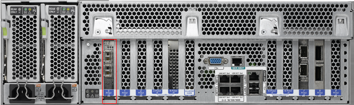
Figure 5-2 Connecting the Optical Cable: Dual Port HBA in Oracle Exalytics In-Memory Machine X3-4
