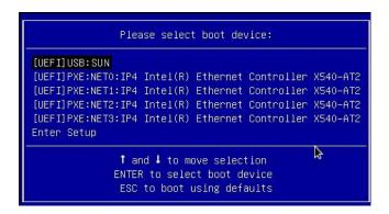
**Note -** The Please Select Boot Device menu that appears in your installation might differ depending on the type of disk controller and other hardware, such as PCIe network cards, installed in your server.
