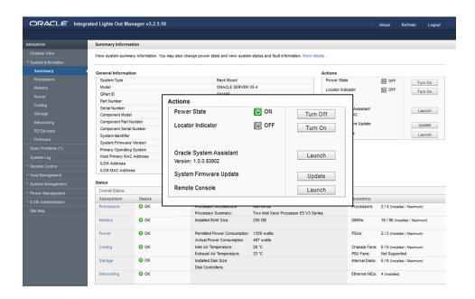
Main power is applied to the server. After a short period, the Power State Off indicator lights green and the Turn On button changes to a Turn Off button.
