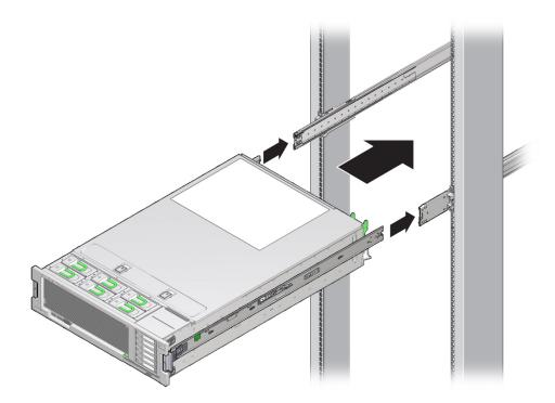
5. Simultaneously push and hold the green slide-rail release buttons on each mounting bracket while you push the server into the rack. Continue pushing
