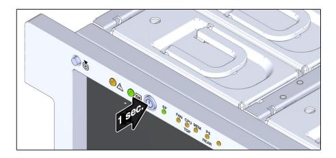
Once main power shuts down, the system enters standby power mode. The OK indicator blinks in standby power mode.
