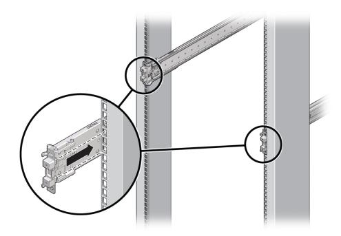
**Note** - The slide assembly mounting pins accommodate either 9.5-mm square mounting holes or M6 round mounting holes. No other mounting hole sizes are supported.
