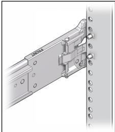
4. (Optional) If you chose to attach the slide-rail assembly with mounting screws and cage nuts, insert the M6 mounting screws through both front and rear slide-rail brackets and rack posts, then secure them with the cage nuts.
