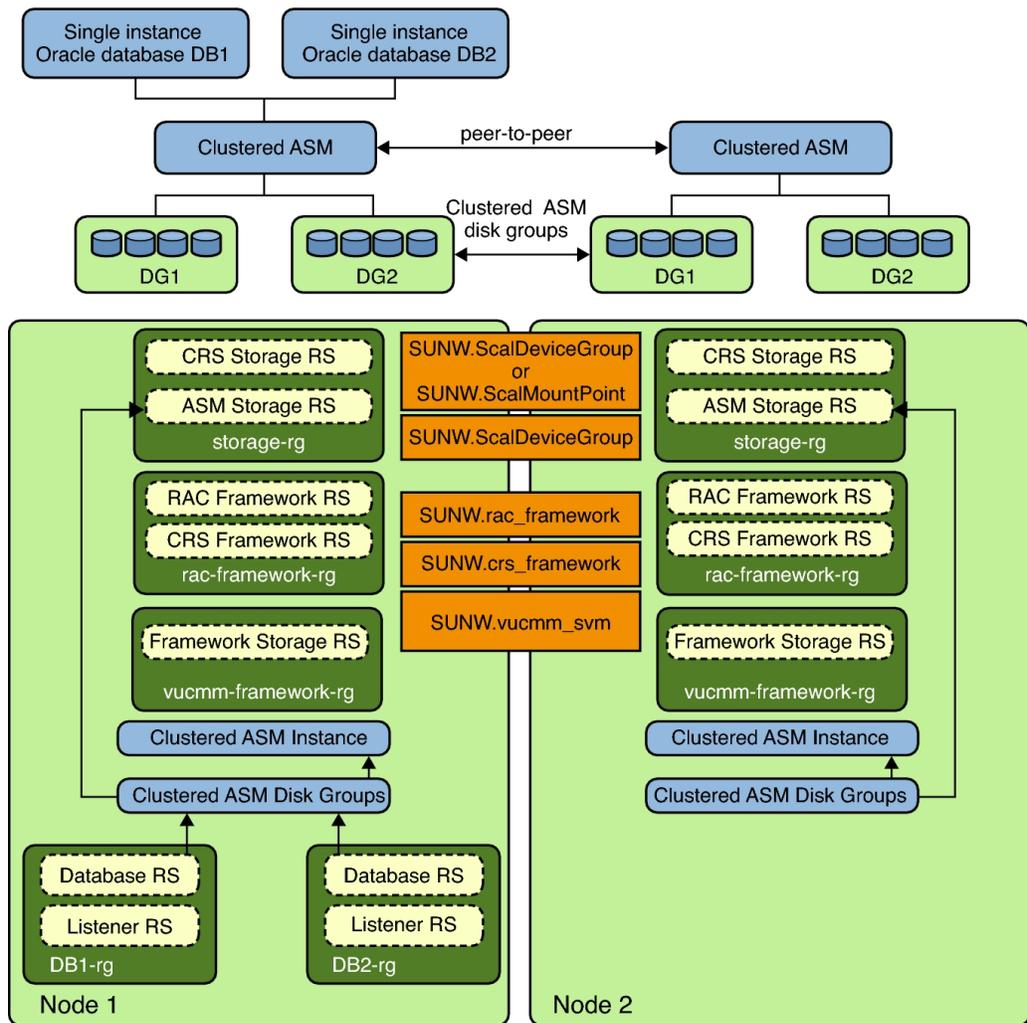
In the following diagram, a single instance Oracle Database DB2 that shares Oracle ASM disk groups DG1 and DG2 is now running on Node2 after a failover of resource groups DB2- rg to Node2. The upper part of the diagram shows the relationships of the Oracle Database instances with the clustered Oracle ASM instances on Node1 and Node2. The clustered Oracle ASM instances manage two Oracle ASM disk groups on both nodes at the same time. The lower part
