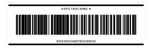
The Intelligent Mail Package Barcode functionality within Documaker generates the barcode symbol. The additional container items can be applied in Documaker Studio using lines, text labels, and variable fields. Note that if Documaker calculates the MOD 10 check digit the check digit value will not be available for inclusion in the field displaying the human readable portion of the barcode.
