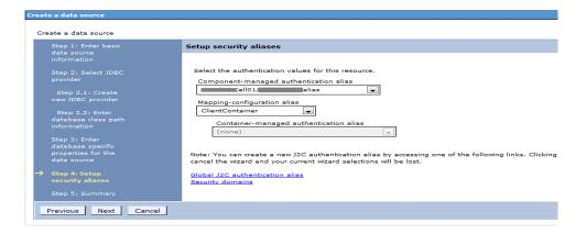
and then save it to the master configuration. Select the data source created and click on test connection.
