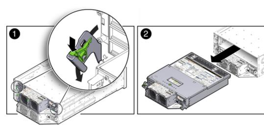
3 Slide the server node to the rear and lift it out of the system [2].
