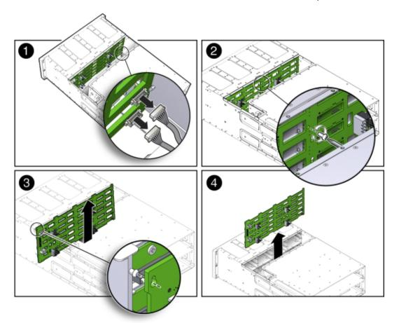
c. Remove the Phillips screw that secures the disk midplane module to the disk drive cage [2].
