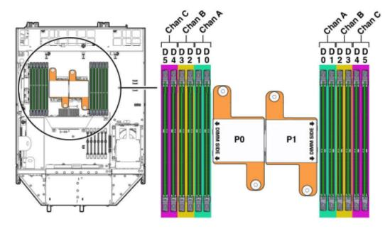
Each processor socket supports three independent memory channels labeled channel A, B, and C, where channel A is closest to the processor socket. Each channel supports two DIMM slots, is controlled by an independent memory controller, and operates independent of the other channels.
