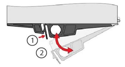
3 Grasp the lever and remove the I/O module.
