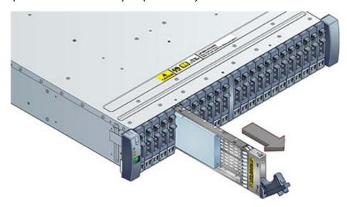
5 Open the drive lever on the replacement drive.
