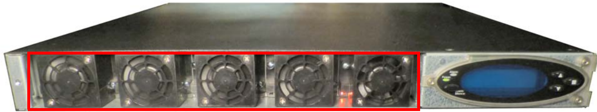
Figure 2 - 11. Intake Fans (shown with front bezel removed)
