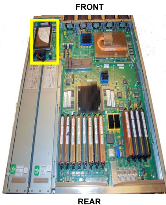
Figure 6 - 125: Location of installed SSD
