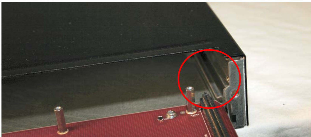
Figure 6 - 106. Aligning the NIU Card with the Chassis Slot Guides
