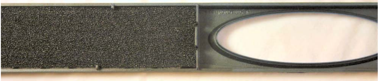
Figure 2 - 36. Acme Packet 4600 Air Filter Behind Front Bezel
