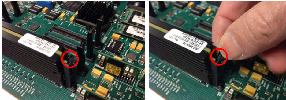
Figure 6 - 117. Releasing the Fastener Holding the Transcoder DSP Module (1 of 2)
