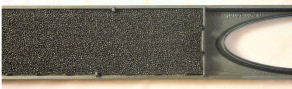
Figure 6 - 138. Air Filter Installed Behind the Front Bezel
