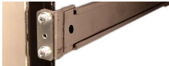
Figure 4 - 57. Installed Slide Rail in a Square-Hole Rack - Front Mount Point
