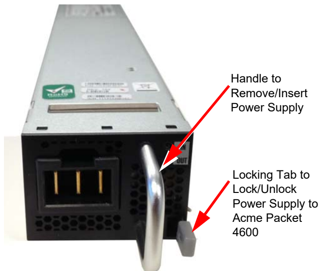
Figure 2 - 34. Acme Packet 4600 DC Power Supply
