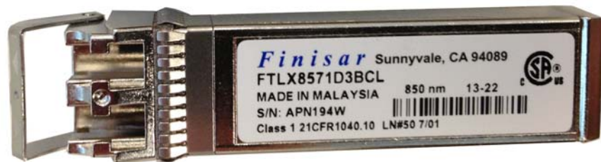
Figure 2 - 26. 10GbE Multi Mode SFP+ Transceiver (Silver Bale Clasp Latch)
