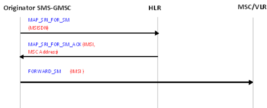
Figure 34: Call flow for Standard MT-SMS Routing
