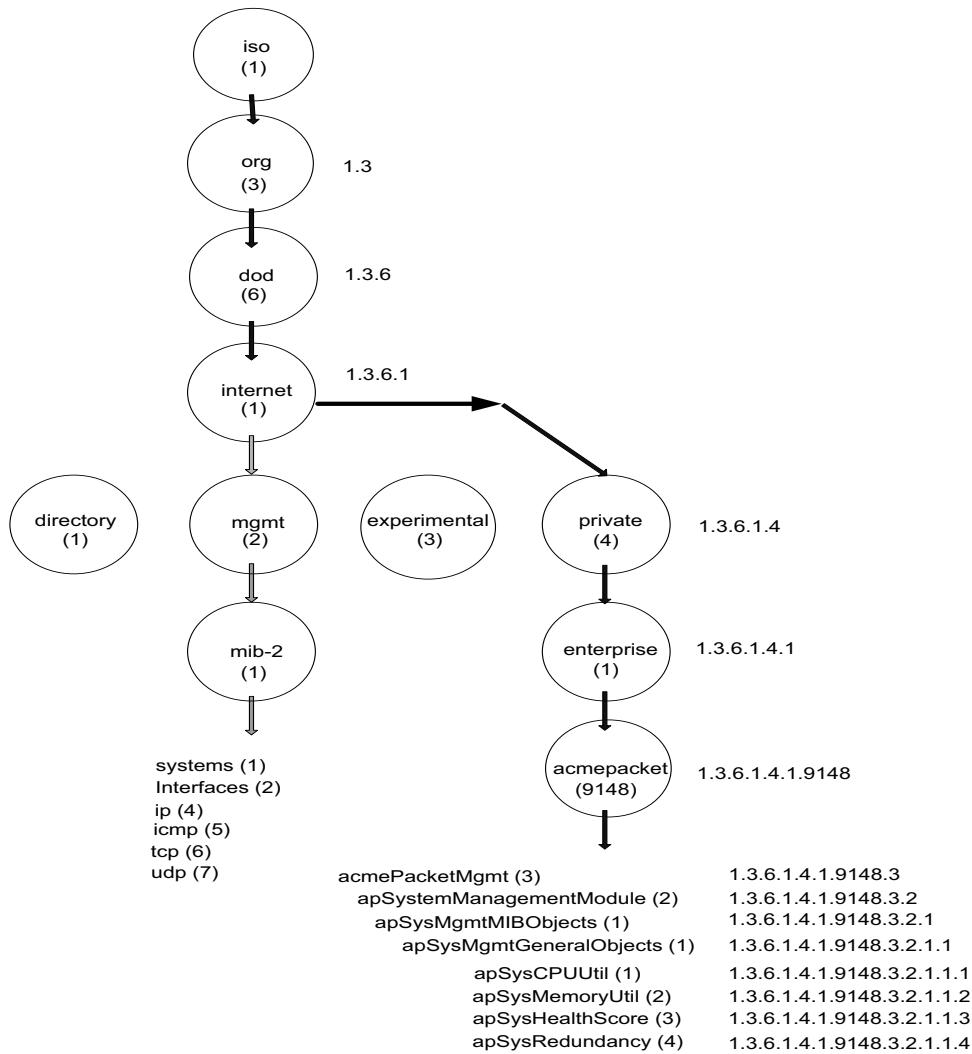
The diagram shows the Acme Packet (Oracle) node has the value 9148; this is Acme Packet's vendor-specific number that uniquely identifies and Acme Packet product MIB. This node is the highest level of the private (proprietary) branch containing Acme Packet managed objects. The number 9148 was assigned to signify Acme Packet's private branch by the Internet Assigned Numbers Authority (IANA).
