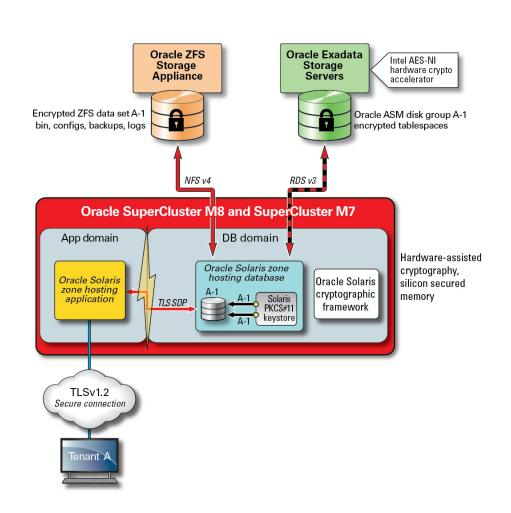
FIGURE 4 Data Protection Provided by the Hardware-Assisted Cryptographic Acceleration and Memory Intrusion Protection
