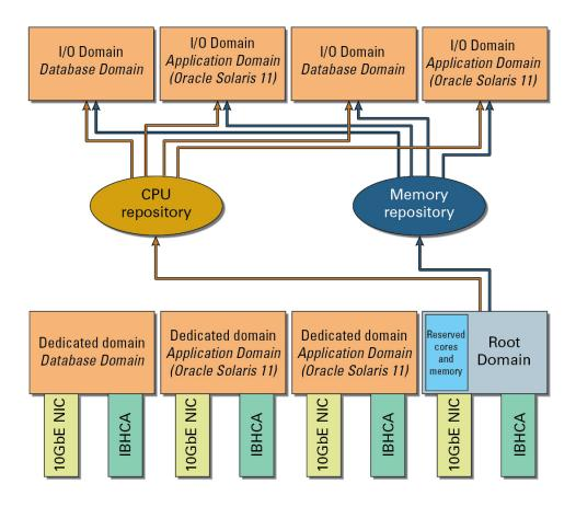
Even though dedicated domains and Root Domains are all shown as equal-sized domains in the preceding figure, that does not mean that CPU and memory resources must be split evenly across all four domains (where each domain is allocated 25% of the CPU and memory resources). Using information that you provide in the Configuration Worksheets, you can
