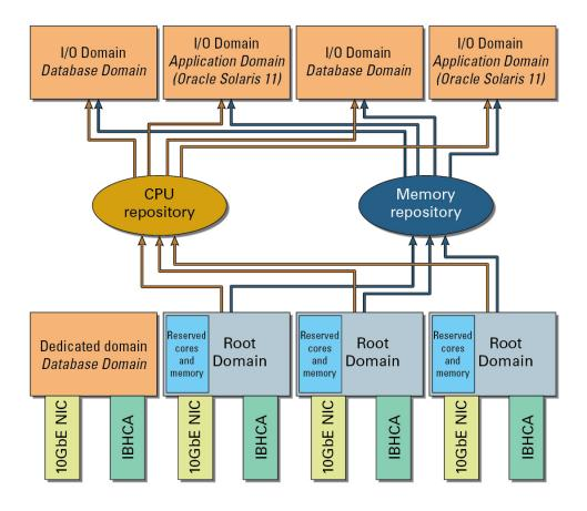
You use the SuperCluster Virtual Assistant to assign the CPU and memory resources to the I/O Domains, based on the amount of CPU and memory resources that you want to assign to each I/O Domain and the total amount of CPU and memory resources available in the CPU and memory repositories. Refer to the I/O Domain Administration Guide for more information.
