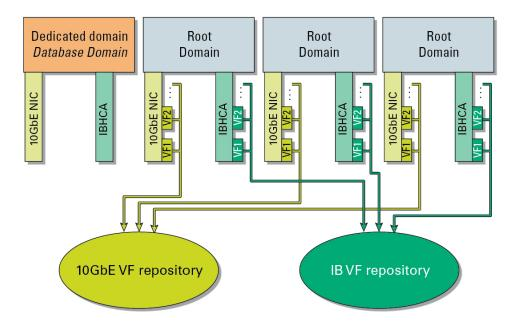
Even though the VFs from each Root Domain are parked in the VF repositories, the VFs are created on each 10GbE NIC and IB HCA, so those VFs are associated with the Root Domain that contains those specific 10GbE NIC and IB HCA cards. For example, looking at the example configuration in the previous graphic, the VFs created on the last (rightmost) 10GbE NIC and IB HCA are associated with the last Root Domain.
