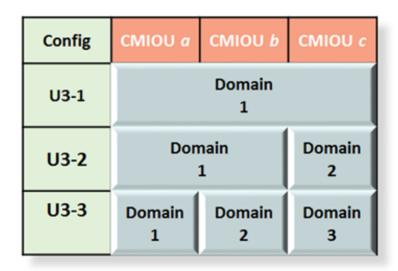
The specific CMIOU number varies, depending on which PDomain is being used as shown in this table.
