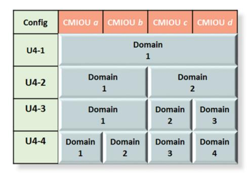
The specific CMIOU number varies, depending on which PDomain is being used as shown in this table.
