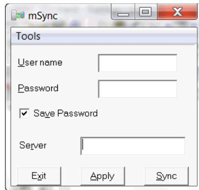
To bring up the mSync GUI, execute `msync.exe` on Win32 and Windows Mobile or `msync` on Linux, which is located in the `/bin` subdirectory under the directory where you installed the mobile client. For Blackberry and Android platforms, start mSync by clicking the mSync application icon.
