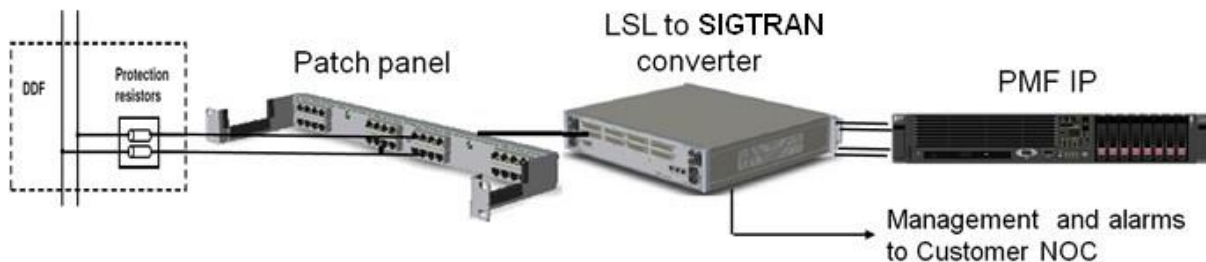
Figure 58 – LSL/HSL to SIGTRAN Converters – connectivity
