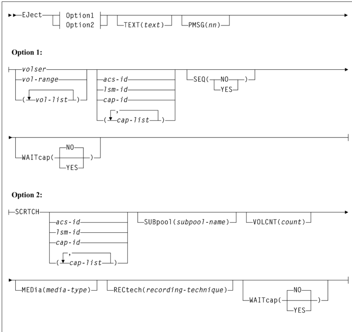
Figure 3–86 Eject command syntax
