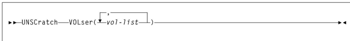
Figure 3–178 UNSCratch command syntax
