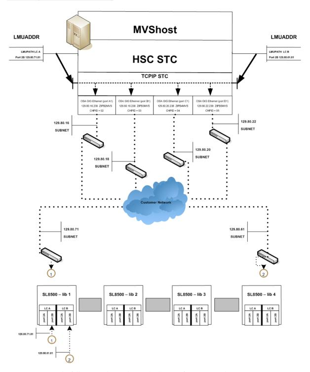
The following rules apply to a dual LC configuration. Both LCs
