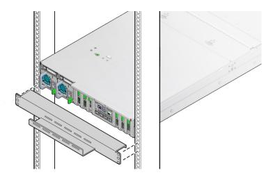
4. Using a No. 2 Phillips screwdriver, secure the bracket to the rack using four 16-mm M6 screws.
