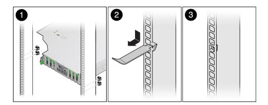
3. Slide the bracket underneath the rear bottom edge of the server chassis with the cable trough facing up, aligning the top holes in the bracket with the first rail holes below the rear panel of the server.
