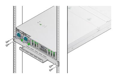
5. If necessary, lay any cables protruding from the server back panel into the cable trough.
