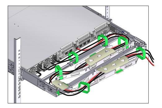
16. Ensure that the secured cables do no extend above the top or below the bottom of the server to which they are attached; otherwise, the cables might snag on other equipment installed in the rack when the server is extended from the rack or returned to the rack.
