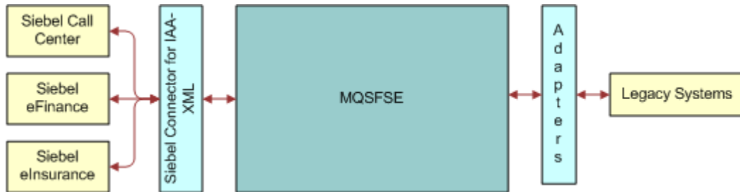
Figure 4. Integration Between Siebel Applications and MQSFSE
