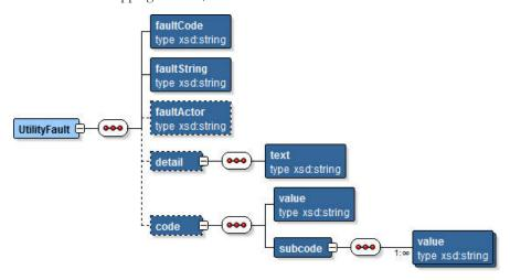
Typically, the faultCode, faultString, faultActor, and detail/text elements will be populated.
