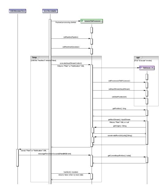
When FA finds a file in the input directory, it instantiates and calls GFP which in turn starts an interaction with the FP. The interaction can be categorized into the following three phases:
