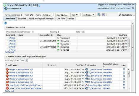
When you click on the instance ID, a new window opens showing the entire process flow. This view is particularly useful in debugging. For instance, clicking on the 1792068 instance in the above image, shows this flow sequence:
