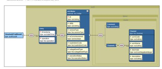
This element is an entry consisting of a timestamp and an Operation. Each entry may have an associated meter object showing what changed.
