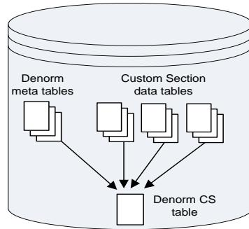
**1 - The data from the denormalization metadata tables is combined with the various Custom Section and Extended Attribute tables in PLM4P and is then pushed into the single table created for the given Custom Section**
